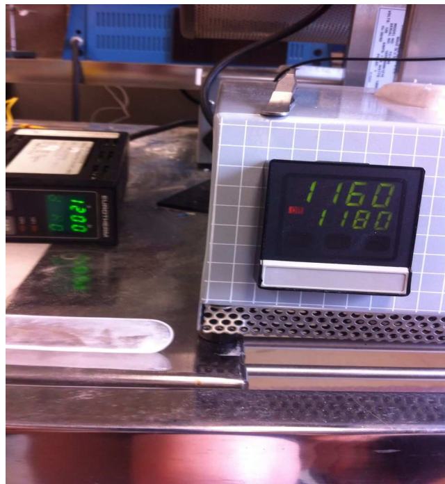
Figure 3.2: Offset temperature of quartz tube furnace. The quartz tube furnace showing the offset between the actual temperature read by thermocouple, setpoint, and read by the furnace.
