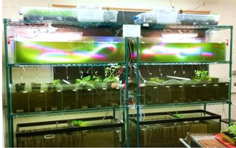
Fig. 6. the experimental aquaponic systems before experimentation began. For the experiment the top terrestrial component was detached and the hydroponic planters were removed.
