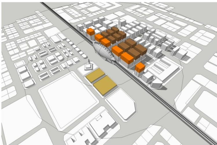
Fig (6-12) 3D visualization of some intensification alternative scenarios generated by transferring the model output to a graphic software (Sketch UP V.4) as a step toward building a full Spatial Decision Support System SDSS.
