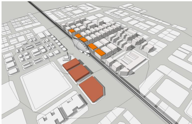
Fig (6-13) 3D visualization of some intensification alternative scenarios generated by transferring the model output to a graphic software (Sketch UP V.4) as a step toward building a full Spatial Decision Support System SDSS.
