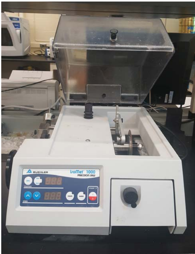
Figure 3.2. Diamond blade Buehler Isomet 1000 precision saw, used to cut sections of embedded rib bone samples for viewing in the SEM.
