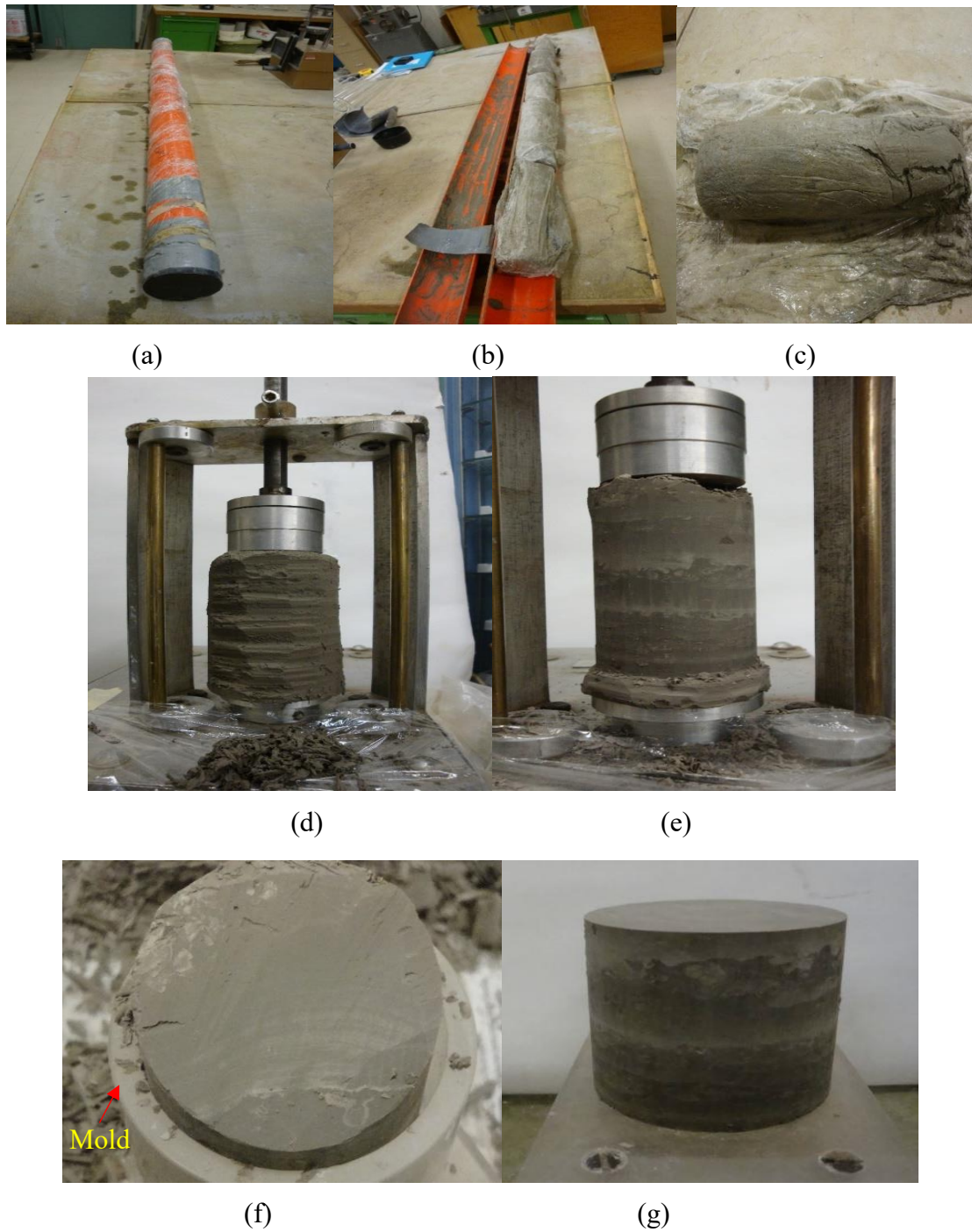
Figure 3-9 Trimming specimen to the proper diameter and length
