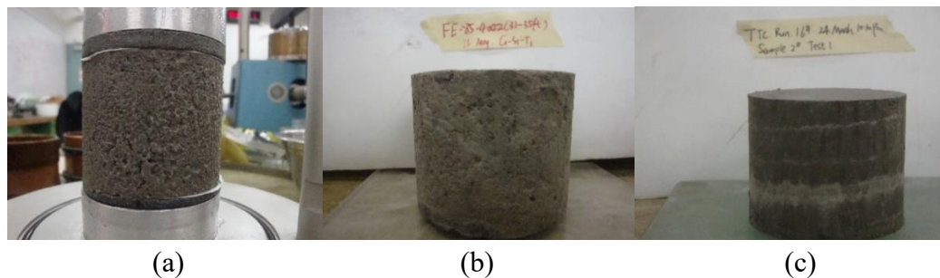
Figure 4-4 Tested materials for making a comparison (a) Homogeneous soil #2004 (b) Heterogeneous soil #4002 (c) Layered soil #5022
