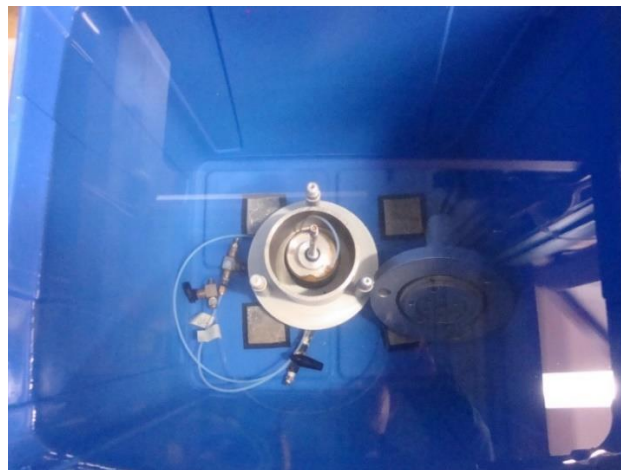
Figure 3-12 Put the triaxial cell together under water to avoid introducing air
