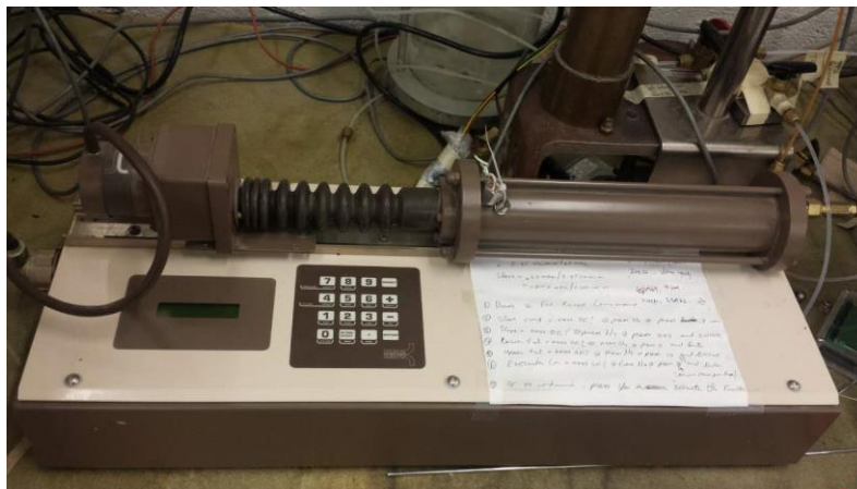
Figure 3-6 GDS digital controller for compliance compensation
