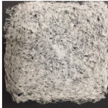
Figure 1.3 The fiber network detached from the glass bead bed (5% SDS, 10% gelatin, 30g/m 2 )
