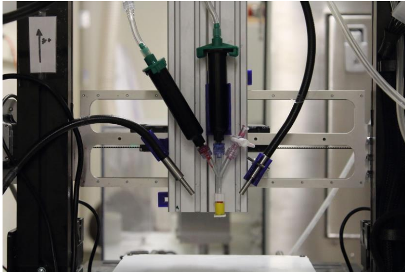
Figure 4.4, A photo of the printhead, the aluminum foil UV protection is not included for clarity, one of the barrels is replaced with an air purge valve.
