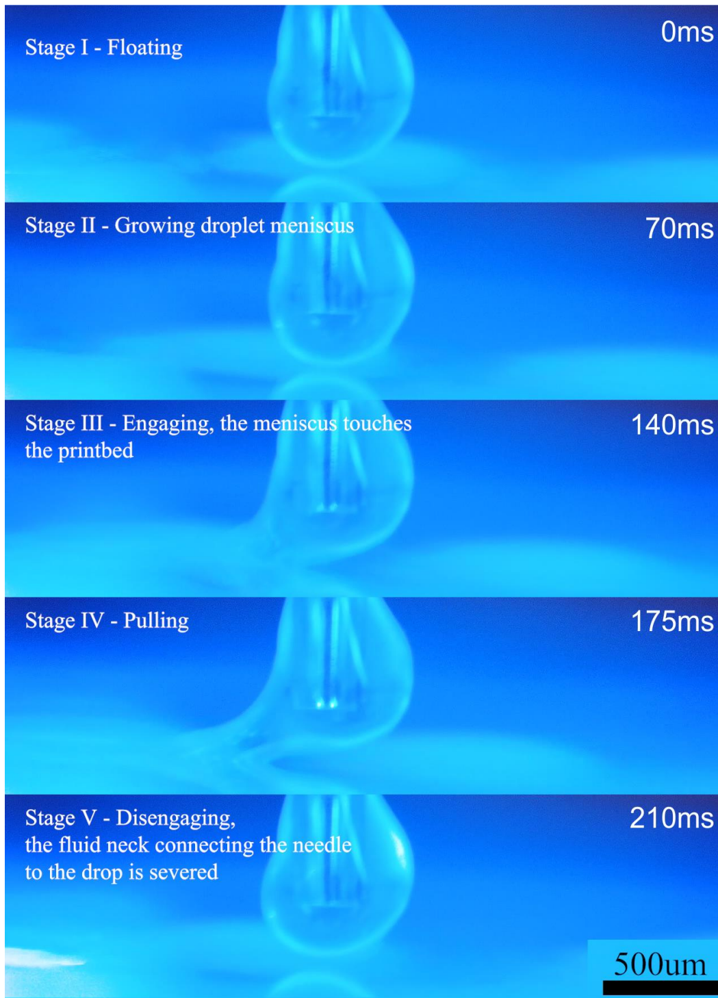
Figure 5.9, A composite from 5 stills showing the stages of the periodic deposition cycle. The large bulb of cured ink on the droplet is the undesired result of capillary flow of the ink up the needle followed by cure from indirect UV. Top right is the time sequence in milliseconds
