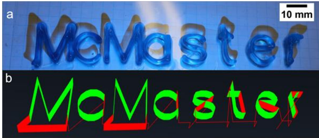
Figure 6.2, a) 3D Printed V31H 'McMaster' sign. b) The toolpath for the above sign. Green path is regular moves, red moves are rapid moves.
