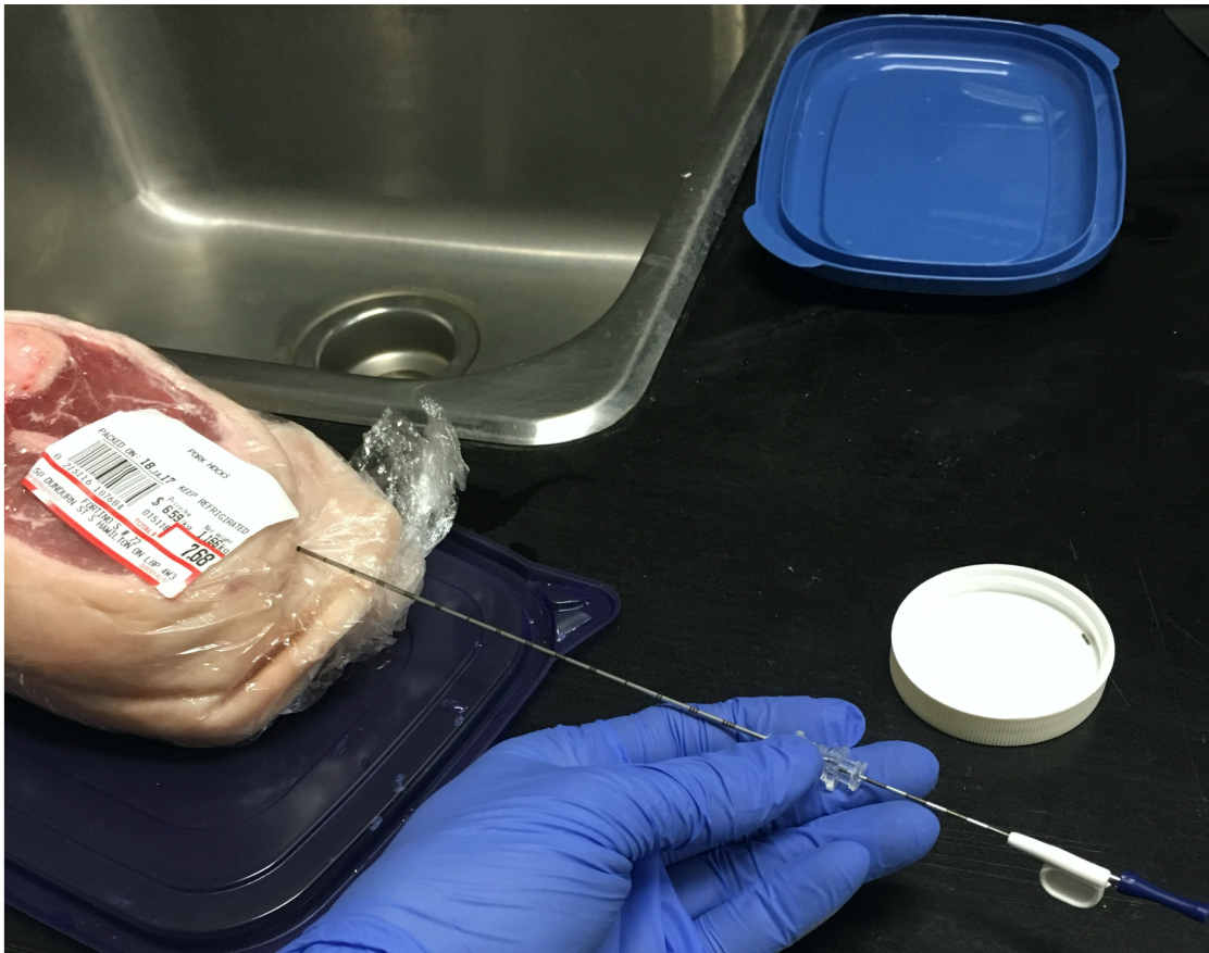
Figure 5.4: Needle Injection of a LDR brachytherapy seed and GFM into porcine tissue. Each seed was inserted approximately 5 cm into the distal end relative to the bone.
