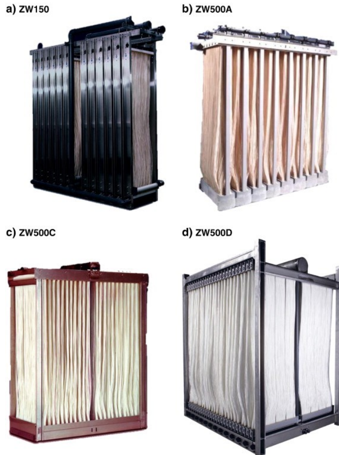
Fig 1.4. Picture demonstration of different ZeeWeed hollow-fiber membrane cassettes (from SUEZ Water Technologies & Solutions) a. ZW150 with 12 modules per cassette (1995); b. ZW500A with 8 modules per cassette (1997); c. ZW500C with 22 modules per cassette (2000); d. ZW500D with 48 modules per cassette (introduced in 2003, improved design presented in 2010). For more information refer to Cote et al. [26] (figure reprinted with permission).
