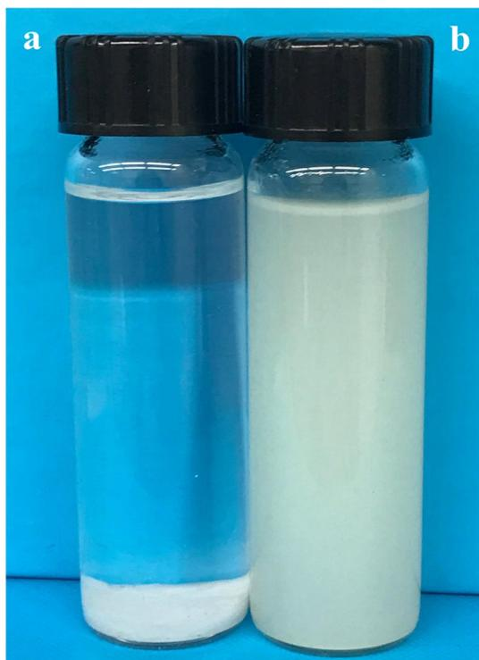
Figure. 5-25. Sedimentation test for  $\text{Al}(\text{OH})_3$ , prepared by (a) precipitation and drying and (b) precipitation and extraction. The suspensions contained 2g/L  $\text{Al}(\text{OH})_3$  and 1g/L CMC in a mixed water-alcohol solvent
