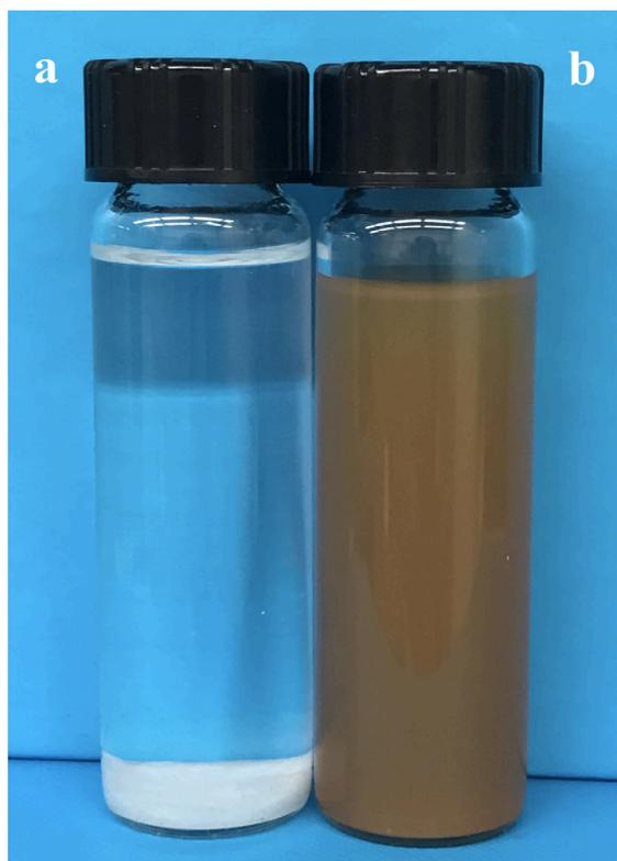
Figure. 5-12. Sedimentation test for  $\text{Al}(\text{OH})_3$ , prepared by (a) precipitation and drying and (b) precipitation and extraction. The suspensions contained 2g/L  $\text{Al}(\text{OH})_3$  and 1g/L QHECE in a mixed water-alcohol solvent
