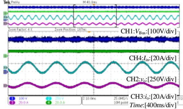
Figure 7.22: Steady-state performance for the fast PI with LCFF case at 500W.
