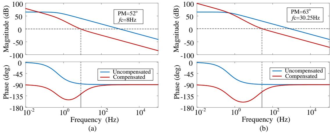
Figure 7.6: Bodeplot of the open-loop and close-loop system: (a) Slow PI case with  $K_p = 6.6e - 3$ ,  $K_i = 0.3$ . (b) Fast PI case with  $K_p = 3e - 2$ ,  $K_i = 3$ .
