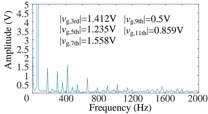
Figure 6.24: FFT analysis of a grid voltage in Marc
