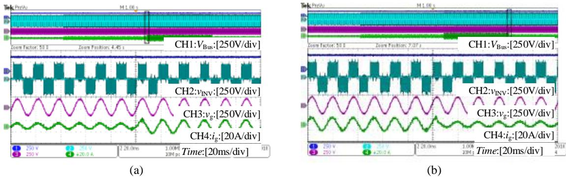
Figure 6.27: Dynamic performance of the grid-tied controller: (a) Half load to full load. (b) Full load to half load.
