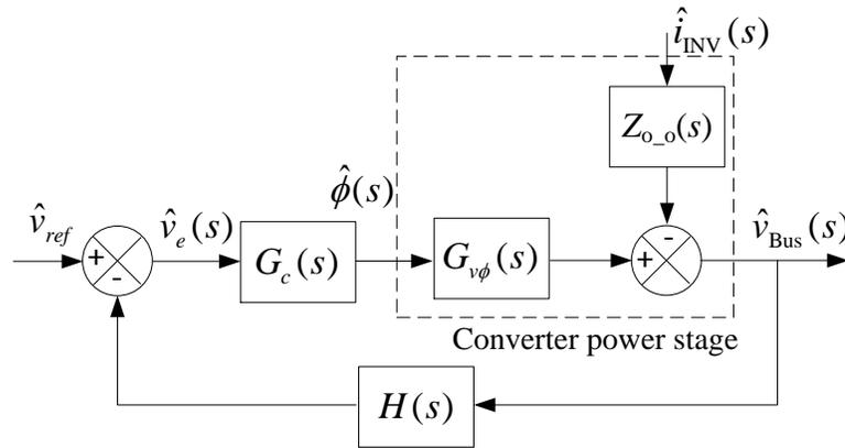
Figure 7.4: Basic control block of three-phase DAB converter.
