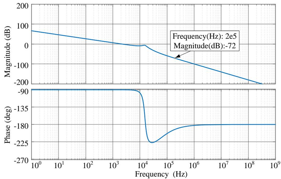
Figure 6.5: Bodeplot of grid-tied transfer function.
