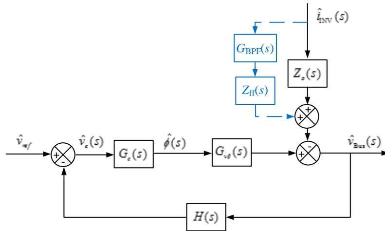
Figure 7.13: Control block with the proposed LCFF path.
