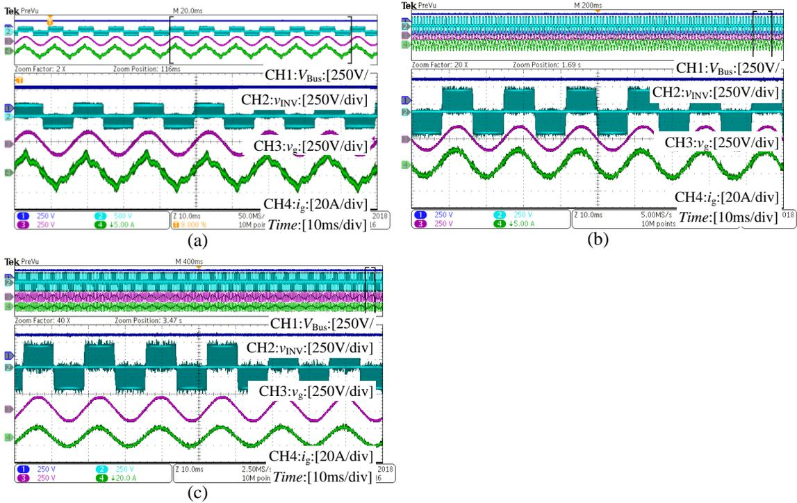
Figure 6.25: 1kW 120V grid-tied mode experimental waveforms: (a) Only PR controller. (b) PR controller with 3rd, 5th HCs. (c) PR controller with 3rd, 5th , 7th, 11th HCs.
