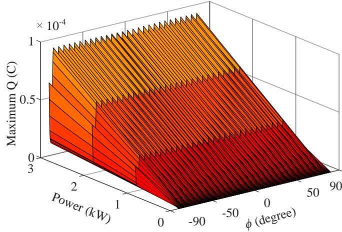
Figure 5.3: Maximum Q for calculating the film capacitor.
