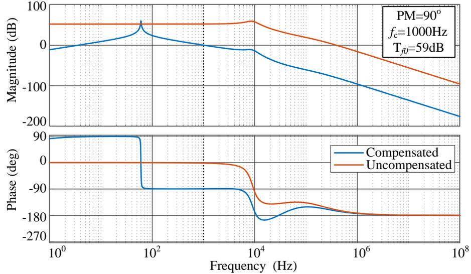
Figure 6.14: Bodeplot of the closed loop standalone inverter.
