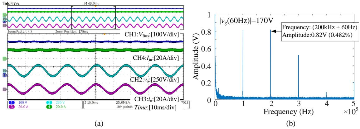
Figure 6.19: 1kW 120V standalone mode experimental results: (a) Waveforms. (b) FFT analysis of the output voltage.
