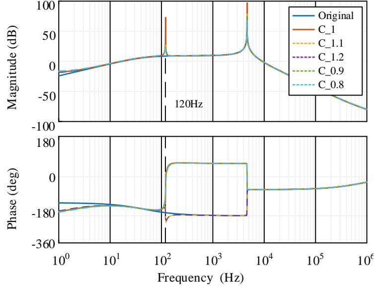
Figure 7.15: Parameter sensitivity analysis of the LCFF method under capacitance error.
