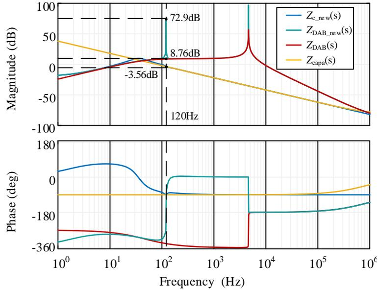
Figure 7.12: Output impedance of the fast PI case with proposed SHC reduction method.
