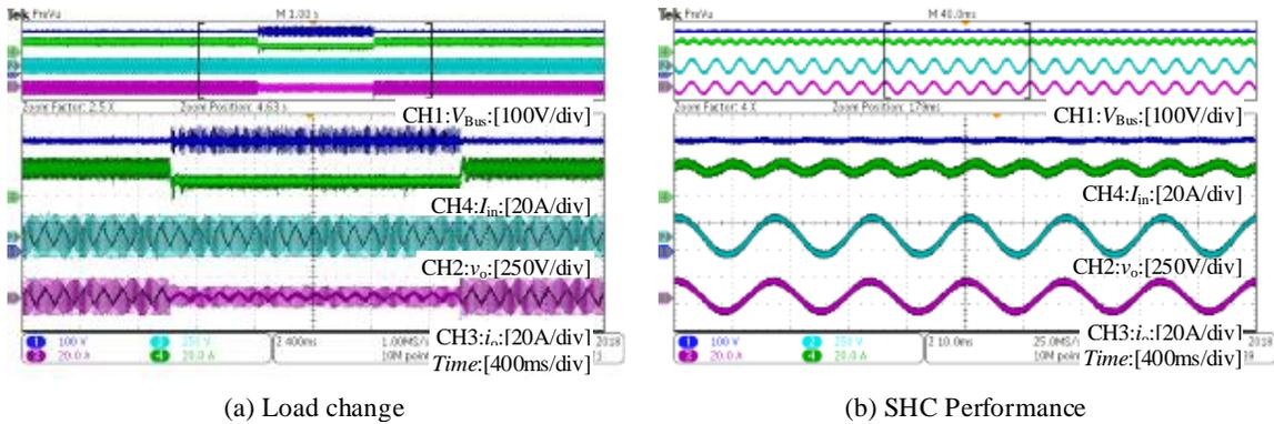
Figure 7.20: Experimental waveforms with the fast PI cast without LCFF control: (a) Load transient response between 1kW and 500W. (b) Steady-state performance.
