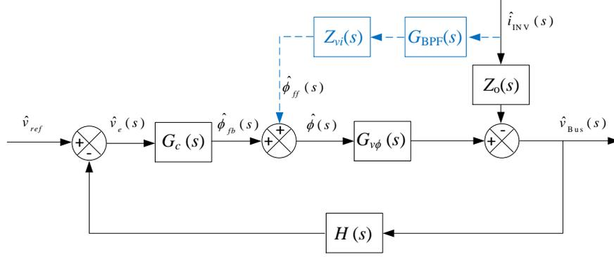
Figure 7.14: Control block with the proposed LCFF path.
