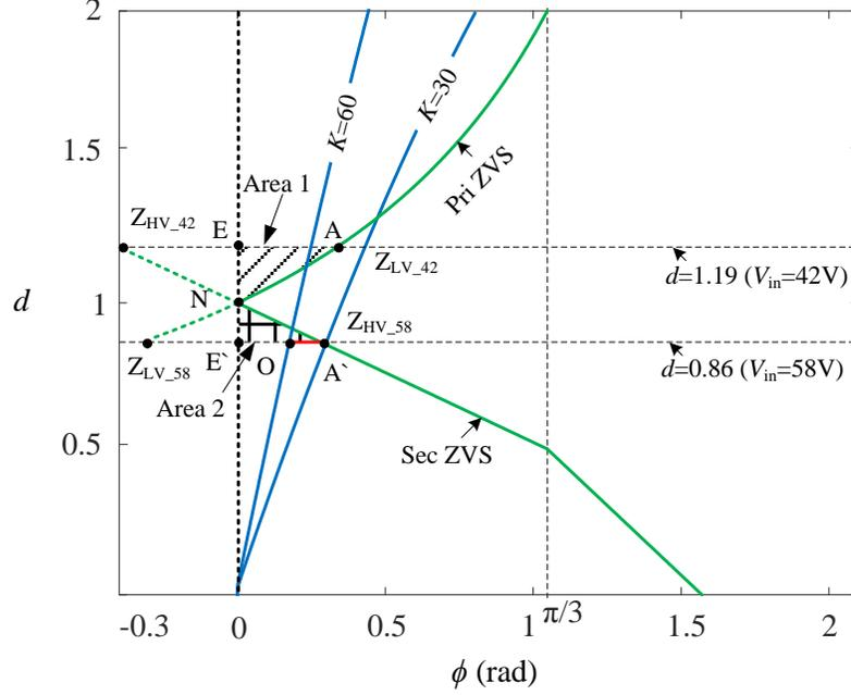
Figure 3.7: Variable switching frequency method analytical analysis.
