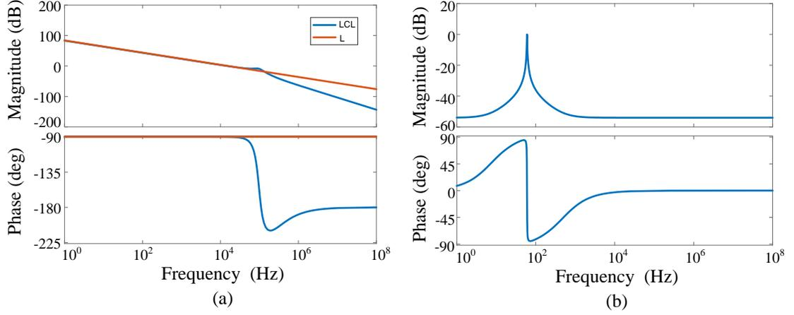
Figure 6.8: Examples for controller design: (a) Comparison between LCL and L filter. (b) Bodeplot of a PR controller.
