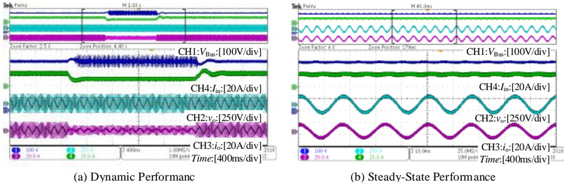
Figure 7.19: Experimental waveforms with the slow PI cast: (a) Load transient response between 1kW and 500W. (b) Steady-state performance.
