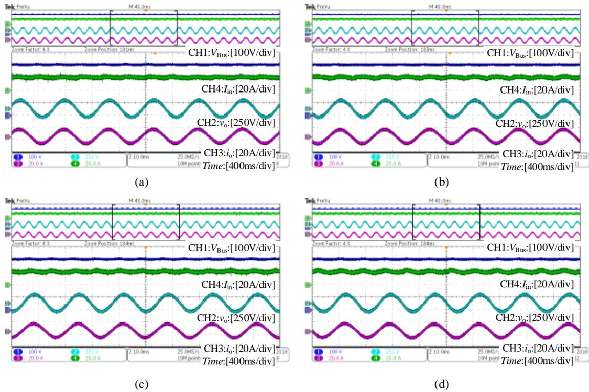
Figure 7.23: Steady-state performance with capacitance error: (a) 110%  $C_2$ . (b) 120%  $C_2$ . (c) 90%  $C_2$ . (d) 80%  $C_2$ .
