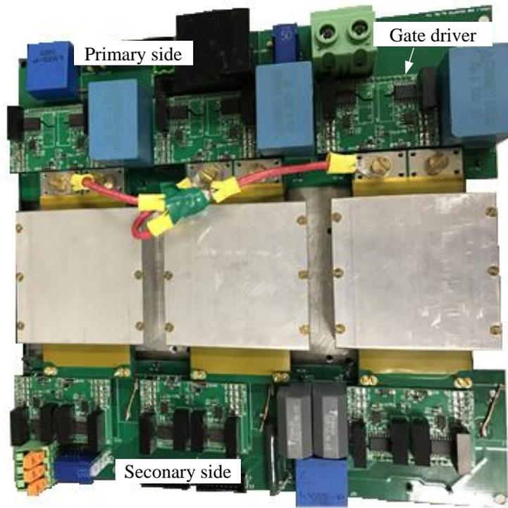
Figure 3.10: Experiment setup of the three-phase DAB converter.
