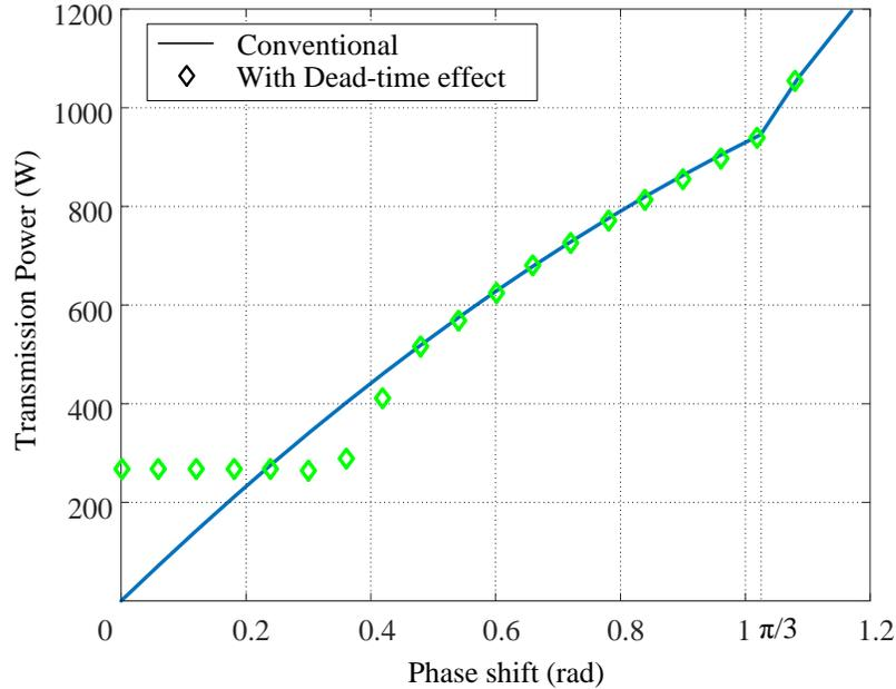
Figure 4.2: Transmission power comparison (Blue solid line: conventional simulated curve with relatively small dead-time; green dots: simulation result with dead-time 0.35 in rad).
