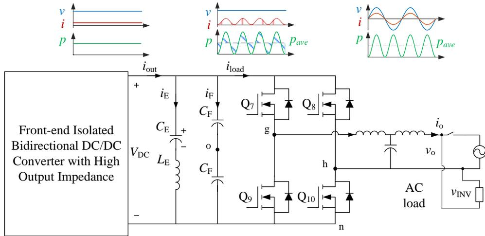
Figure 5.1: Downstream single-phase inverter with hybrid capacitor bank.
