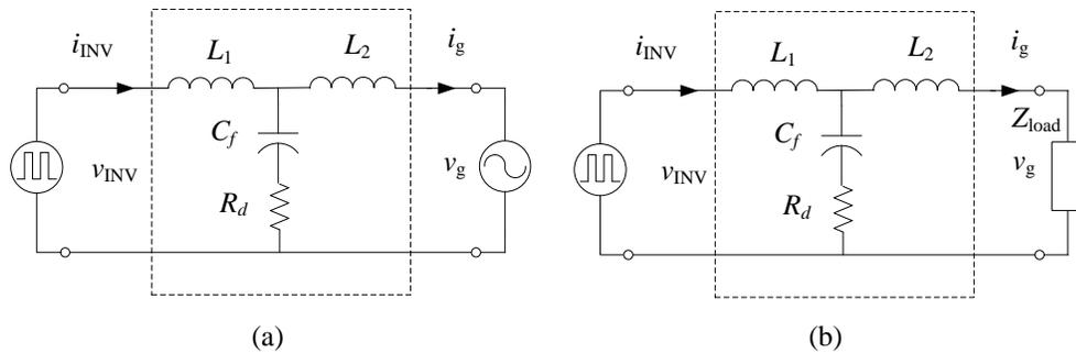
Figure 6.2: Two port network of the single-phase inverter: (a) Grid-tied mode. (b) Standalone mode.
