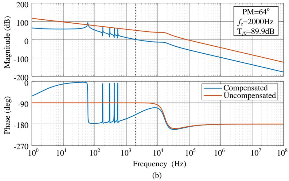
Figure 6.11: A PR controller with multiple HC: (a) Control block with multi-HC. (b) Bodeplot.
