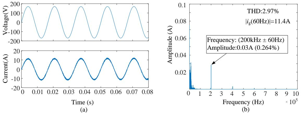
Figure 6.17: 1kW 120V grid-tied mode simulation results: (a) Waveforms. (b) FFT analysis of the grid current.
