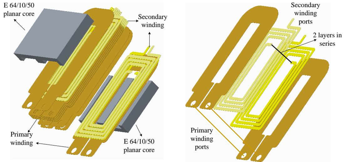
Figure B.6: Terminology and winding stack arrangement of the applied transformer in (Cui Ying, 2017).
