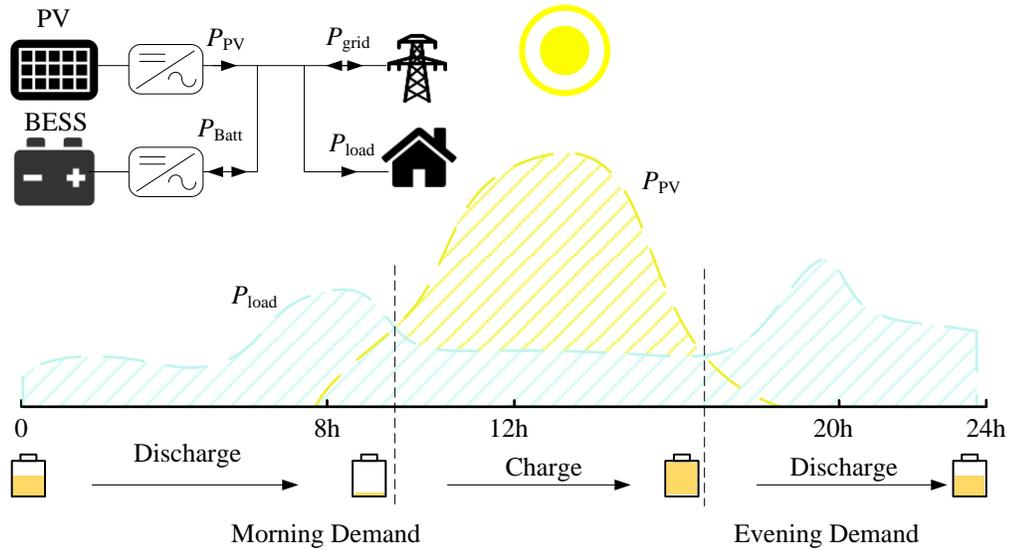
Figure 1.1: Illustration for battery energy storage system in residential microgrid.
