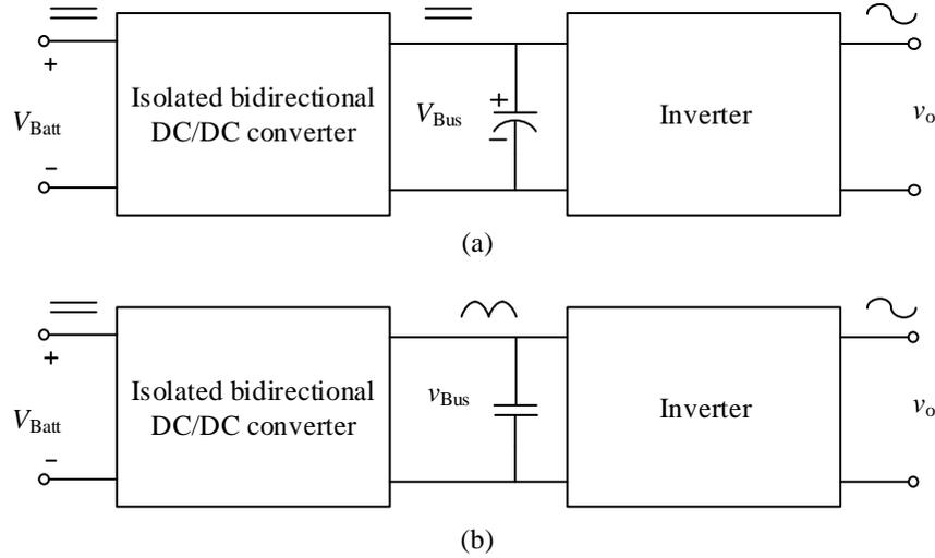
Figure 2.1: Topology evaluation of two-stage isolation bidirectional DC/AC inverter: (a) Stable DC bus voltage. (b) Variable DC bus voltage.
