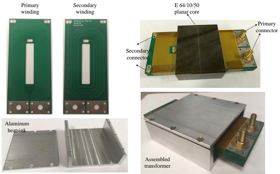
Figure B.7: PCB winding and assembled planar transformer in (Cui Ying, 2017).
