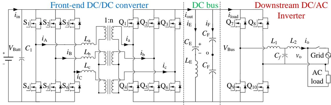
Figure 2.10: Proposed topology for the isolated battery-driven grid interface with the three-phase DAB converter.
