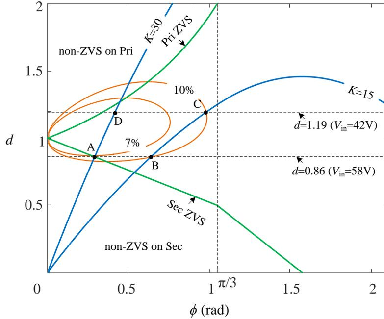
Figure 3.3: Design diagram of the three-phase DAB converter.
