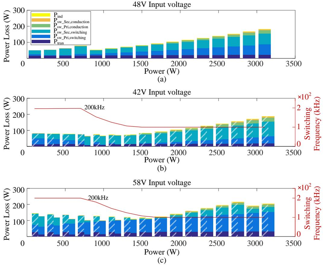
Figure 3.9: Power loss breakdown of the variable switching frequency strategy with different input voltage level. Shaded area represents the power loss breakdown of the 100kHz original operation.
