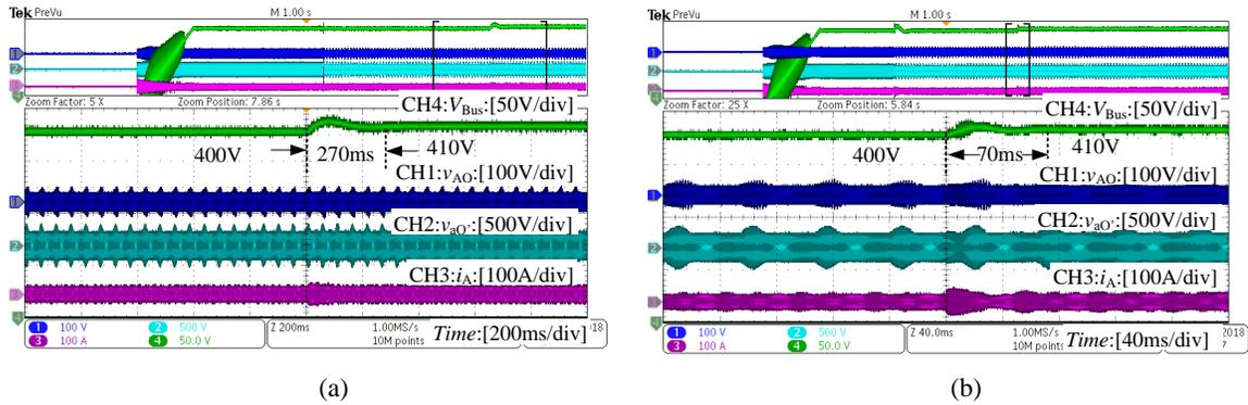
Figure 7.8: Experimental results of step response from 400V to 410V: (a) Slow PI case. (b) Fast PI case.
