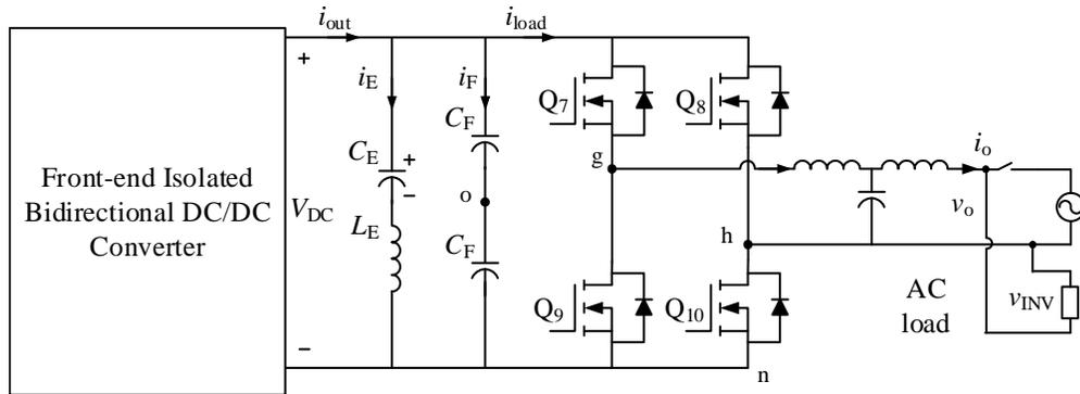
Figure 2.7: Downstream single-phase inverter with hybrid capacitor bank.
