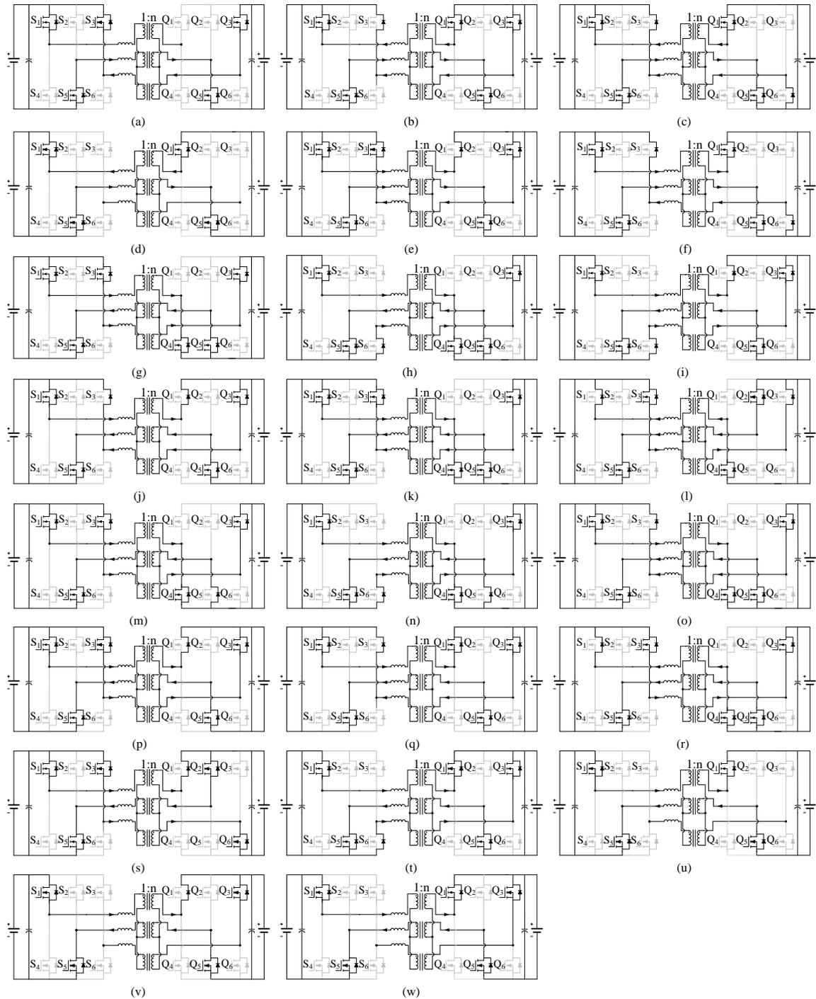
Figure 4.5: Equivalent circuits of the three-phase DAB converter for the dead-time effect analysis.
