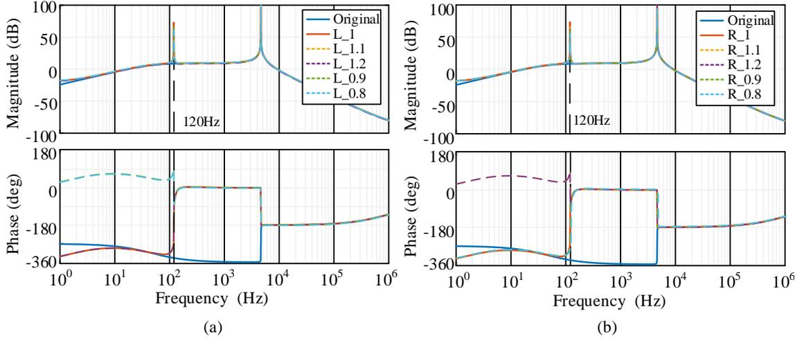
Figure 7.16: Parameter sensitivity analysis of the LCFF method: (a) under  $L_k$  error. (b) under  $R_{load}$  error.
