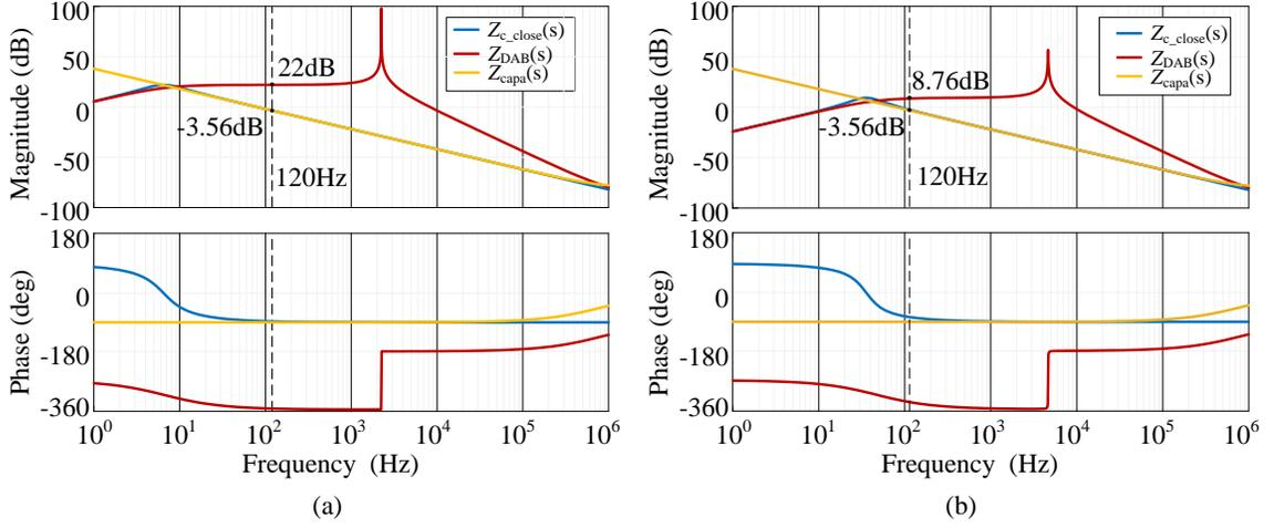
Figure 7.10: Closed-loop output impedance comparison: (a) Slow PI case. (b) Fast PI case.
