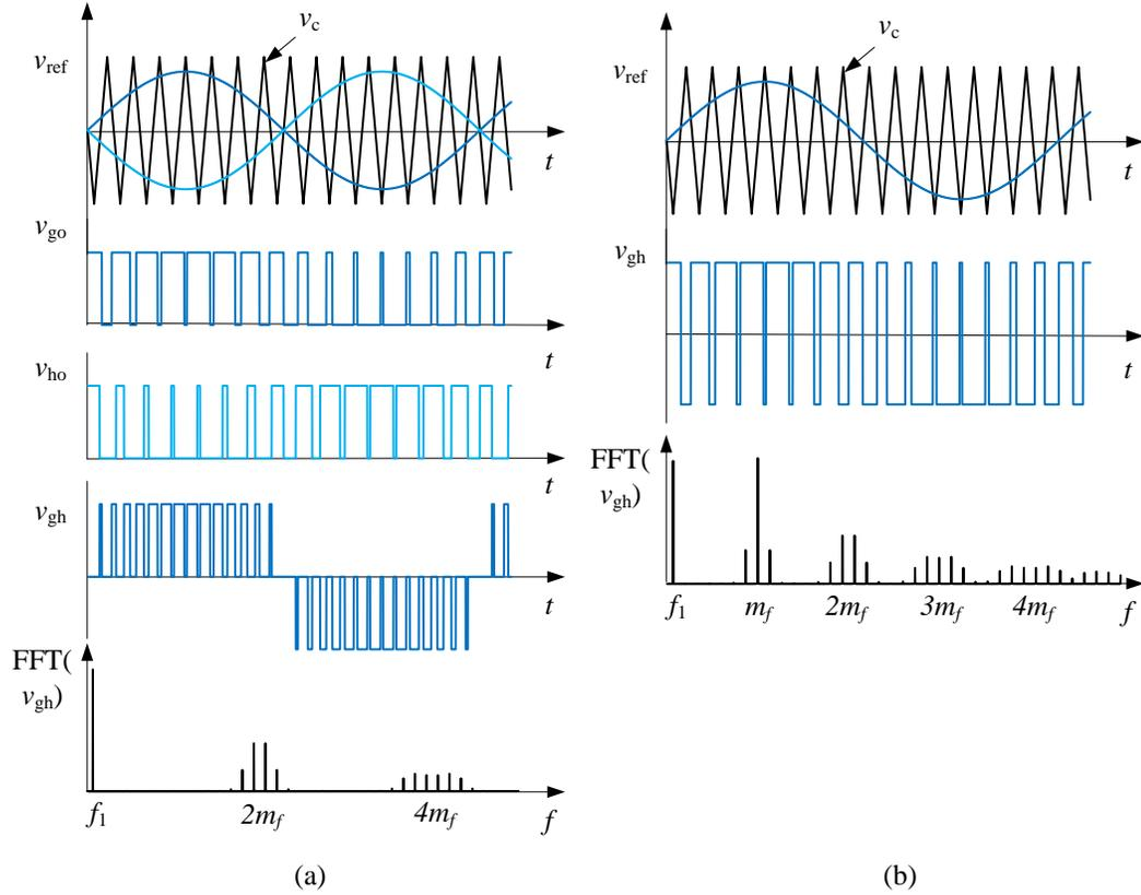
Figure 2.9: Harmonics comparison between the unipolar and bipolar SPWM for single-phase inverter: (a) Unipolar SPWM. (b) Bipolar SPWM.
