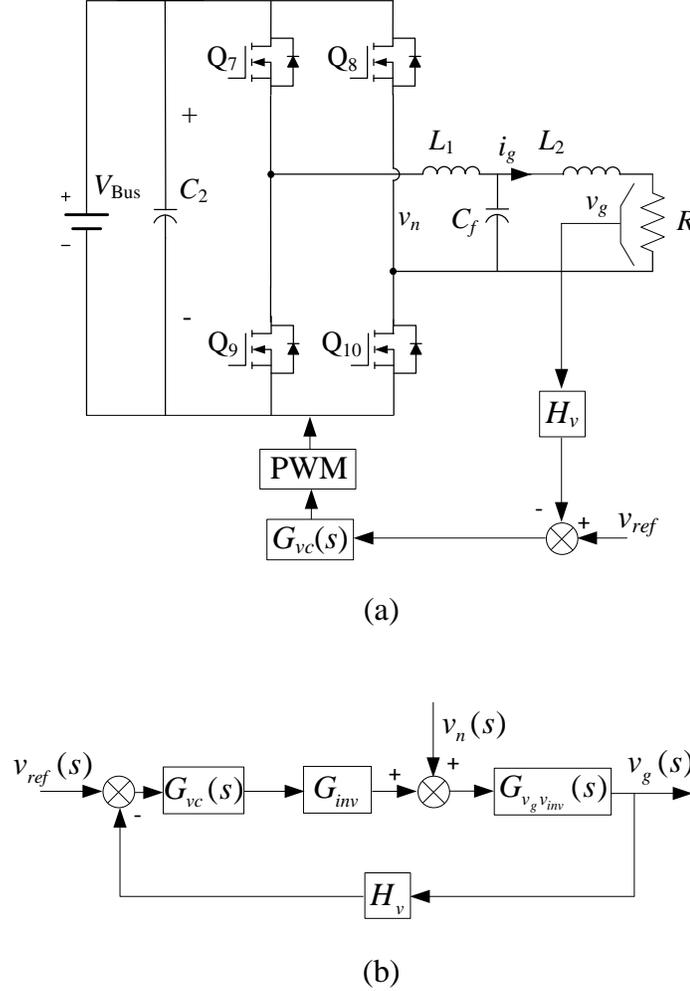
Figure 6.12: Standalone LCL inverter with controller. (a) Configuration of the LCL inverter with controller. (b) Control block diagram of the grid-tied LCL inverter.
