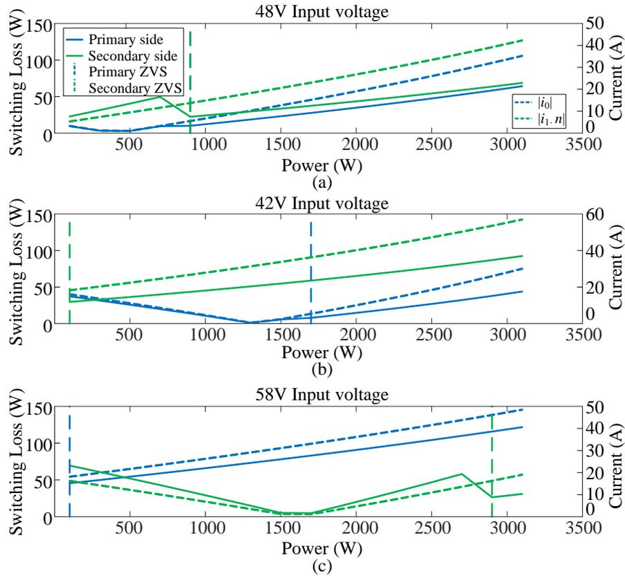
Figure 3.6: Switching loss and the instantaneous current analysis with different input voltage level: (a) 48V input voltage. (b) 42V input voltage. (c) 58V input voltage.
