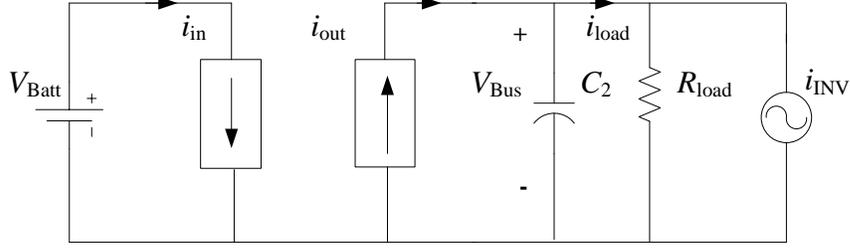
Figure 7.3: Averaged model of the three-phase DAB converter.
