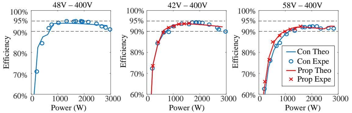
Figure 3.12: Theoretical and experimental efficiency comparison between constant switching frequency operation and variable switching frequency operation.
