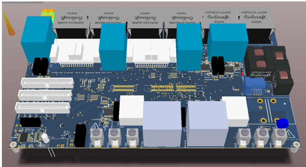
Figure B.8: 3D PCB model of single-phase inverter with controller interface.
