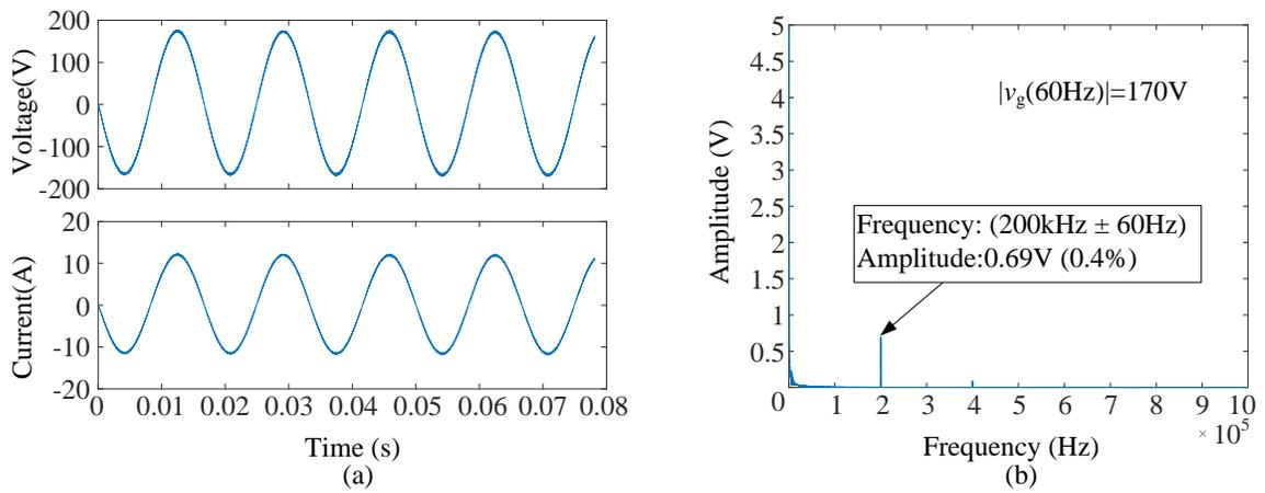
Figure 6.15: 1kW 120V standalone mode simulation results: (a) Waveforms. (b) FFT analysis of the output voltage.
