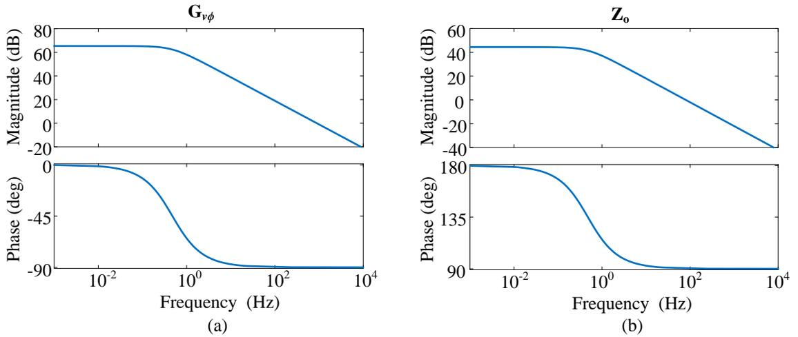
Figure 7.5: Bodeplot of transfer function: (a) phase-shift to voltage transfer function. (b) Output impedance of the front-end converter.
