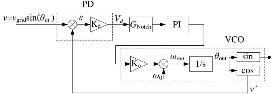
Figure 6.10: Phase locked loop basic structure.
