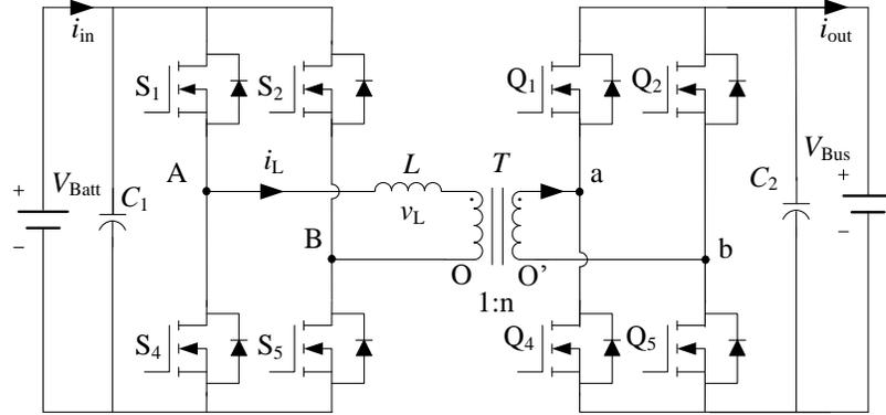
Figure 2.2: Illustration of single-phase DAB converter.
