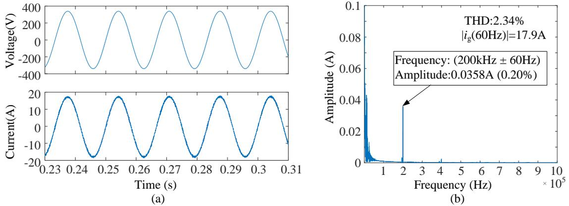
Figure 6.18: 3kW 240V grid-tied simulation results: (a) Waveforms. (b) FFT analysis of the grid current.
