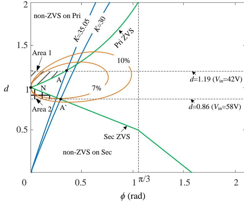
Figure 3.8: Variable switching frequency strategy operation principle.
