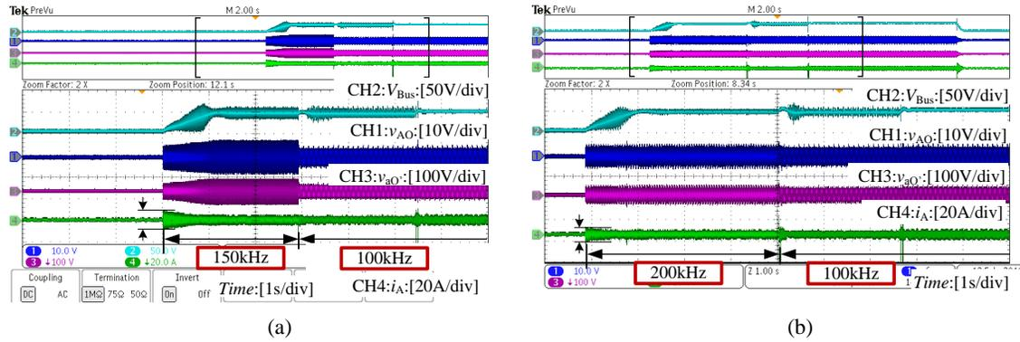
Figure B.12: Transformer current impact comparison during soft-start with difference switching frequency: (a) 150kHz soft-start. (b) 200kHz soft-start.
