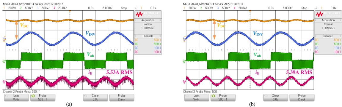
Figure 5.8: Experimental verification of the current sharing method: (a) no add-on  $L_E$ ; (b)  $L_E = 3.3\mu\text{H}$ .
