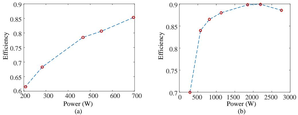
Figure 6.22: Efficiency map of the system: (a) 1kW 120V. (b) 3kW 240V
