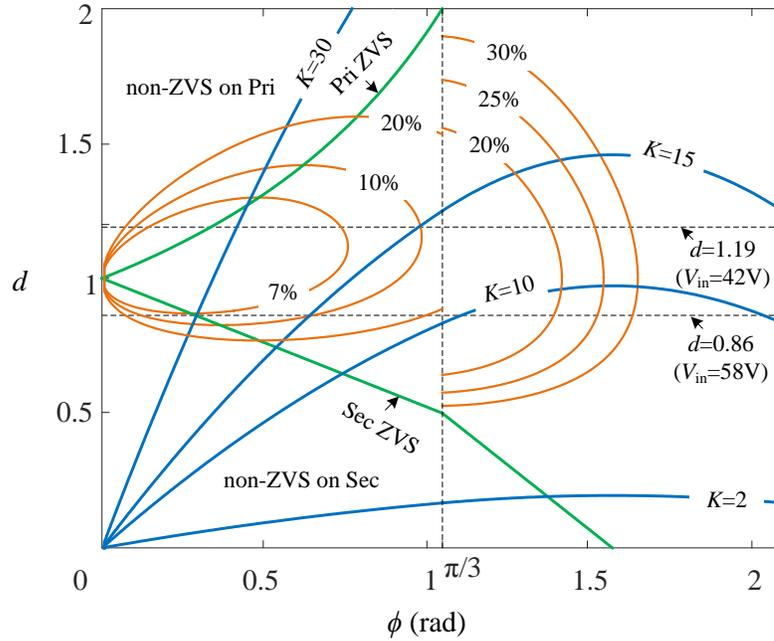
Figure 3.2: Operation illustration of the three-phase DAB converter: blue lines represent  $K$  value; green lines represent the ZVS conditions; orange lines represent the back-flow power ratio.
