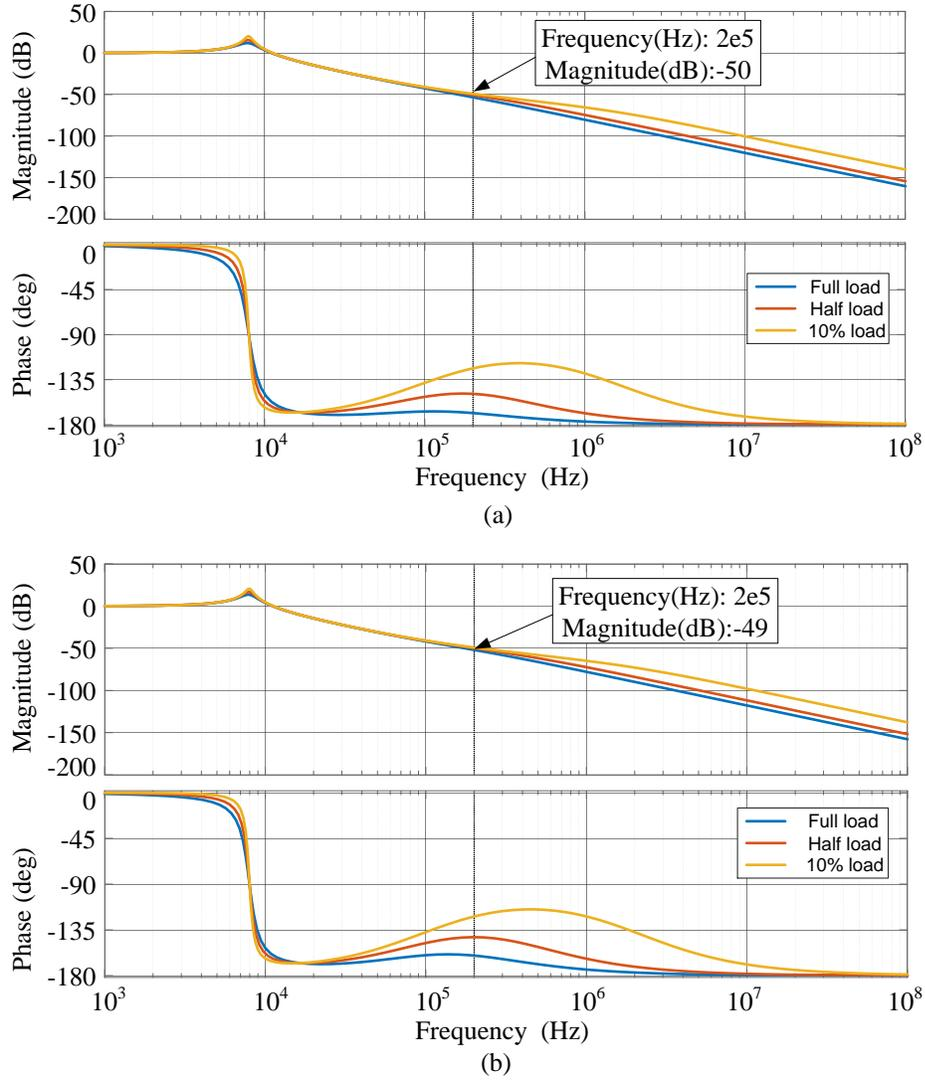
Figure 6.6: Bodeplot of standalone transfer function: (a) 120V case. (b) 240 case.
