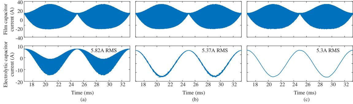
Figure 5.6: Current sharing performance: (a)  $L_E = 10\text{nH}$ ; (b)  $L_E = 3.3\mu\text{H}$ ; (c)  $L_E = 1.25\text{mH}$ .
