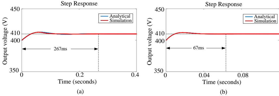
Figure 7.7: Step response of the controller comparison between analytical and simulation results: (a) Slow PI case. (b) Fast PI case.
