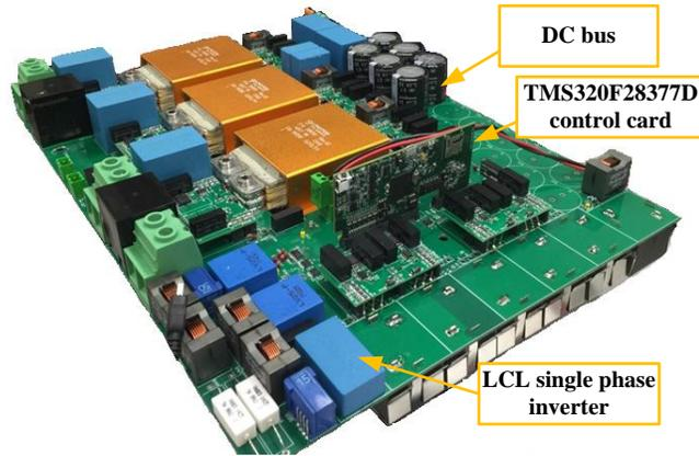
Figure 5.7: Experiment setup for hybrid capacitor bank.
