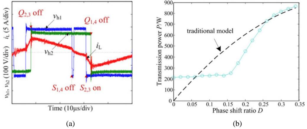
Figure 2.6: Dead-time effect phenomena observed in experimental waveforms of single-phase DAB converter: (a) Voltage Polarity Reversal Phenomenon. (b) Phase Drift Phenomenon. (Zhao *et al.*, 2014b).
