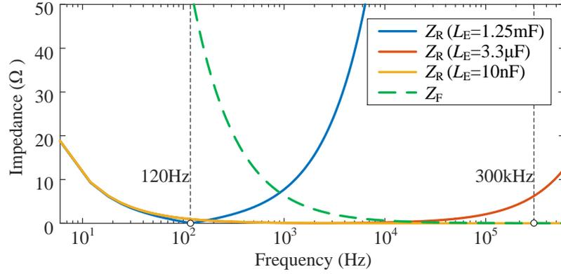
Figure 5.4: Impedance of the resonant filter and film capacitor.
