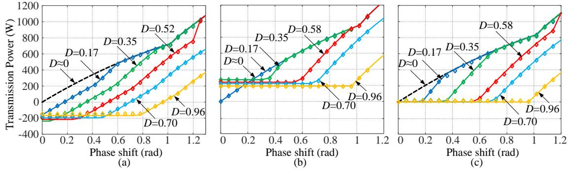
Figure 4.8: Transmission power of the three-phase DAB converter with different dead-time: (a) Boost state; (b) Buck state; (c) Matching state. (Solid line: Theoretical results with dead-time effect; Dash line: Conventional results; Diamond mark: Experimental results).
