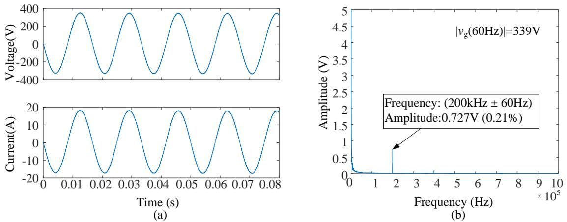
Figure 6.16: 3kW 240V standalone mode simulation results: (a) Waveforms. (b) FFT analysis of the output voltage.
