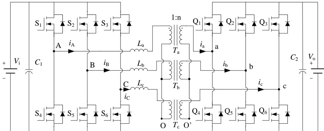
Figure 2.4: Illustration of three-phase DAB converter.
