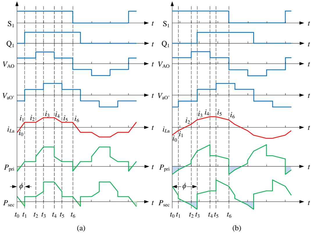
Figure 2.5: Operation waveforms of three-phase DAB converter: (a) $0-\pi/3$  (b) $\pi/3-2\pi/3$ .
