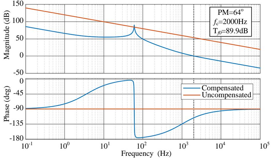
Figure 6.9: Bodeplot of the closed-loop grid-tied inverter.
