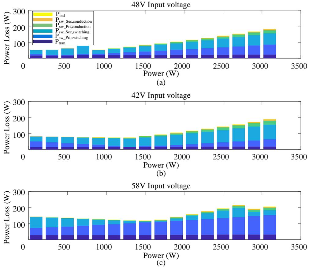
Figure 3.5: Power loss breakdown with constant switching frequency operation in different input voltage level: (a) 48V input voltage. (b) 42V input voltage. (c) 58V input voltage.
