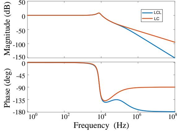
Figure 6.13: Comparison between LCL and L filter for standalone mode.
