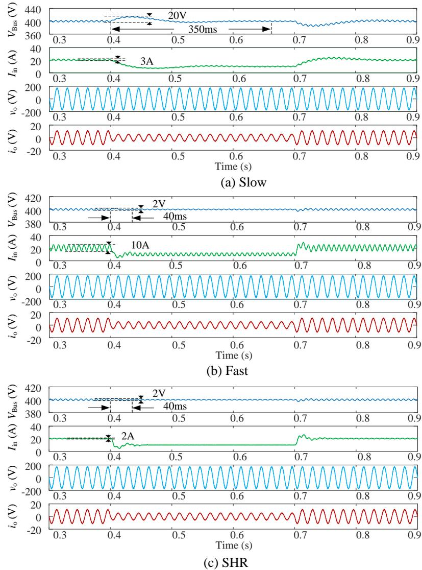
Figure 7.17: Simulation results: (a) the slow PI case. (b) the fast PI without LCFF case. (c) the fast PI with SHR case.
