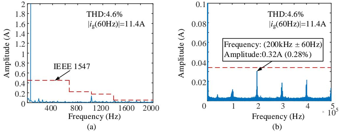
Figure 6.26: FFT analysis of the grid current for 1kW 120V grid-tied mode experimental results: (a) Low frequency. (b) High frequency.
