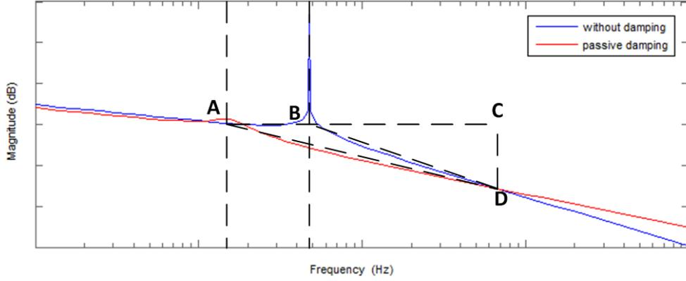
Figure 6.3: Comparison of grid-tied transfer function of LCL between with damping and without damping.
