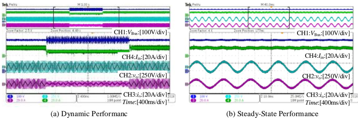
Figure 7.21: Experimental waveforms with the fast PI cast with LCFF control: (a) Load transient response between 1kW and 500W. (b) Steady-state performance.
