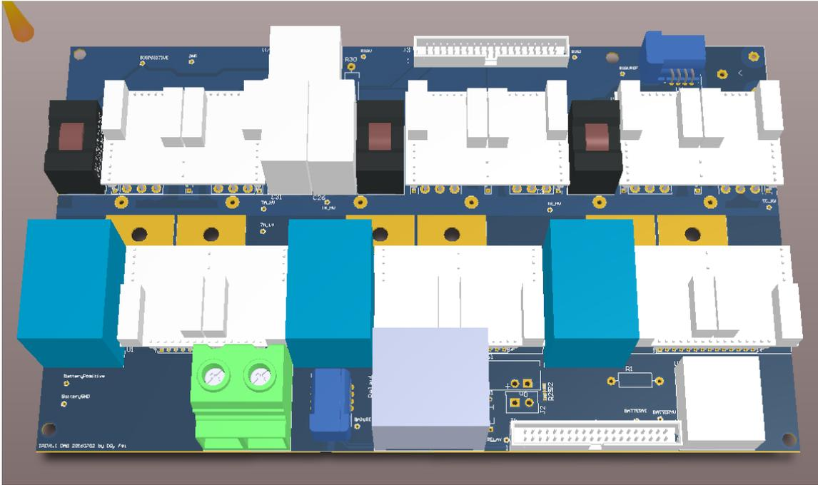
Figure B.5: 3D PCB model of the DAB part in Prototype 2.
