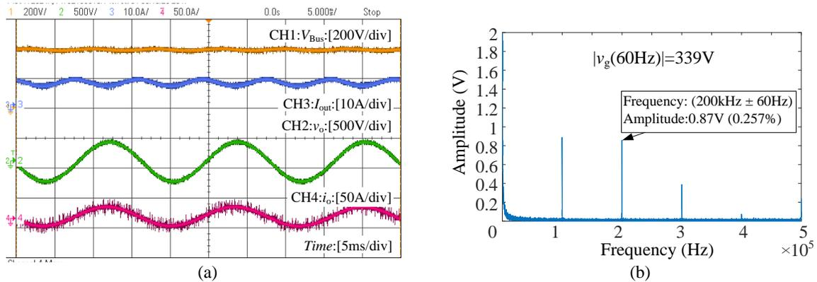
Figure 6.20: 3kW 240V standalone mode experimental results: (a) Waveforms. (b) FFT analysis of the output voltage.
