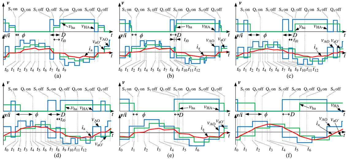
Figure 4.4: Operation waveforms for Buck state.
