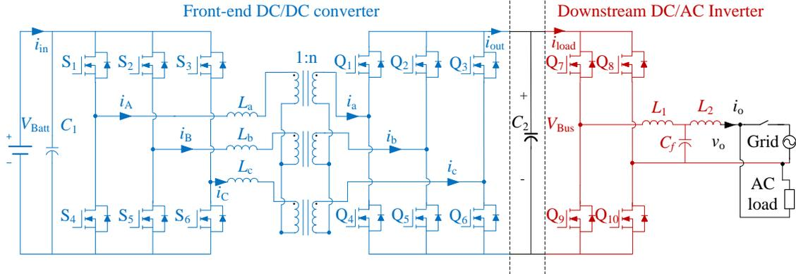
Figure 7.1: A three-phase DAB based IBDGI with downstream single-phase inverter.
