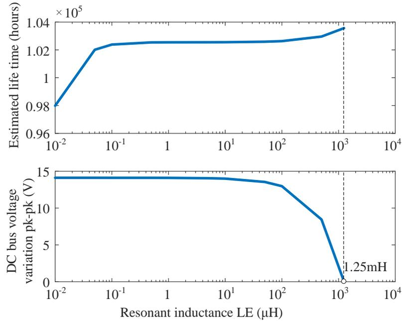
Figure 5.5: Estimated lifetime of the electrolytic capacitor and DC-bus voltage variation with different resonant inductance  $L_E$ .
