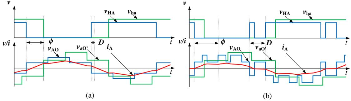
Figure 4.1: Operation waveforms of three-phase DAB converter: (a) Conventional, (b) Dead-time effect (simulation condition: dead-time in rad is 0.70; phase shift in rad is 0.48.)
