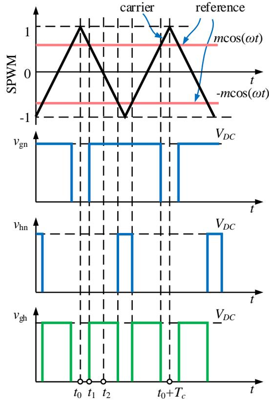
Figure 5.2: Unipolar SPWM modulation illustration.
