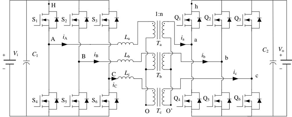
Figure 3.1: Topology of the three-phase DAB converter.
