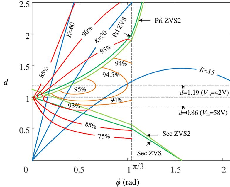
Figure 3.4: Design verification diagram of the converter: blue lines represent K value; dark green lines represent the rough ZVS conditions; light green lines represent the strict ZVS conditions; orange lines represent the efficiency within ZVS zone; red lines are the efficiency curves losing ZVS.
