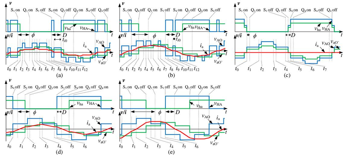
Figure 4.6: Operation waveforms for Matching state.
