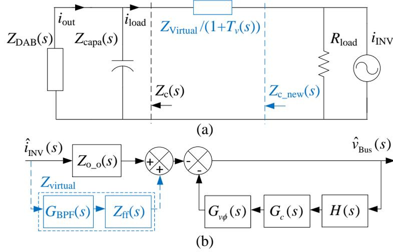
Figure 7.11: Illustration of the virtual impedance idea: (a) Equivalent circuit. (b) Control block with virtual impedance.
