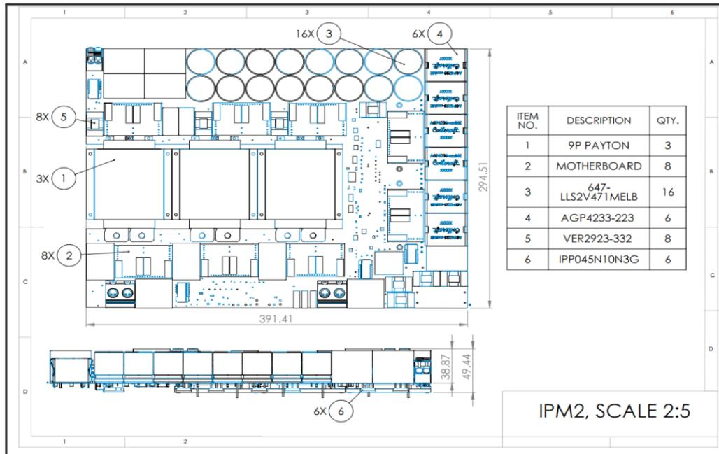
Figure B.2: Size of the Prototype 1 3D model.
