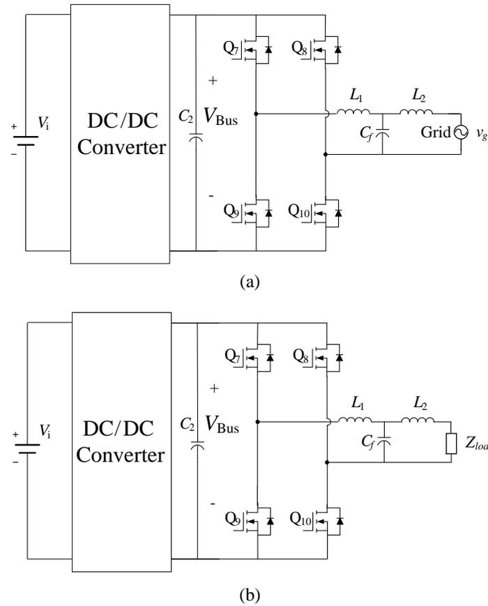
Figure 6.1: The downstream single-phase inverter: (a) Grid-tied mode. (b) Standalone Mode.
