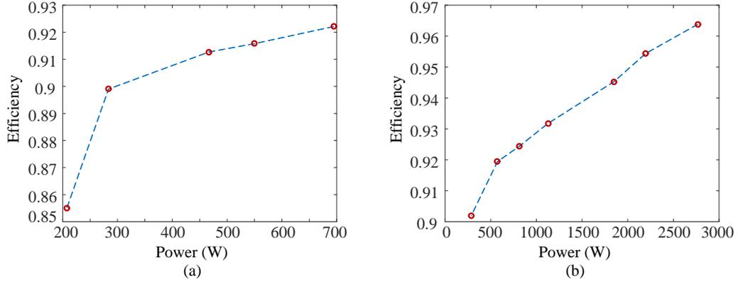
Figure 6.21: Efficiency map of the single-phase inverter: (a) 1kW 120V. (b) 3kW 240V
