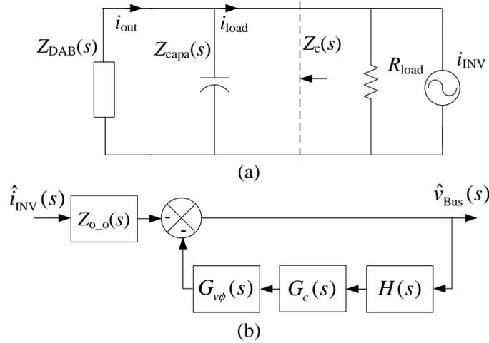
Figure 7.9: Equivalent circuit from output impedance view: (a) Equivalent circuit. (b) Control block with virtual impedance.
