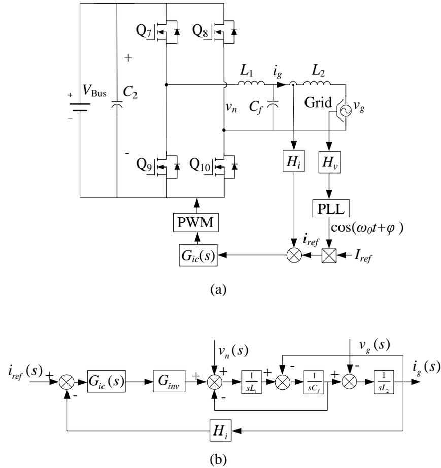
Figure 6.7: Grid-tied LCL inverter with controller: (a) Configuration of the LCL inverter with controller. (b) Control block diagram of the grid-tied LCL inverter.
