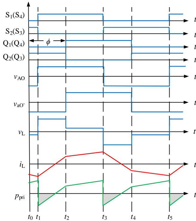
Figure 2.3: Operation waveforms of single-phase DAB converter.
