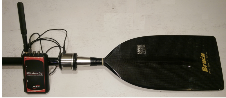
Figure 3.5: Photo of the load cell system attached to the Braca paddle and blade, along with the wireless transducer.
