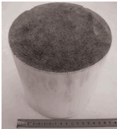
Figure 1.2: Honeycomb structure of the substrate
