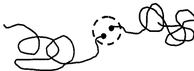
Scheme 1.2: Schematic demonstrating the molecular process involved in bimolecular termination
