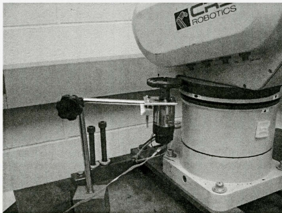
Figure 4-4: External encoder reading angle of the F3 Joint 1
