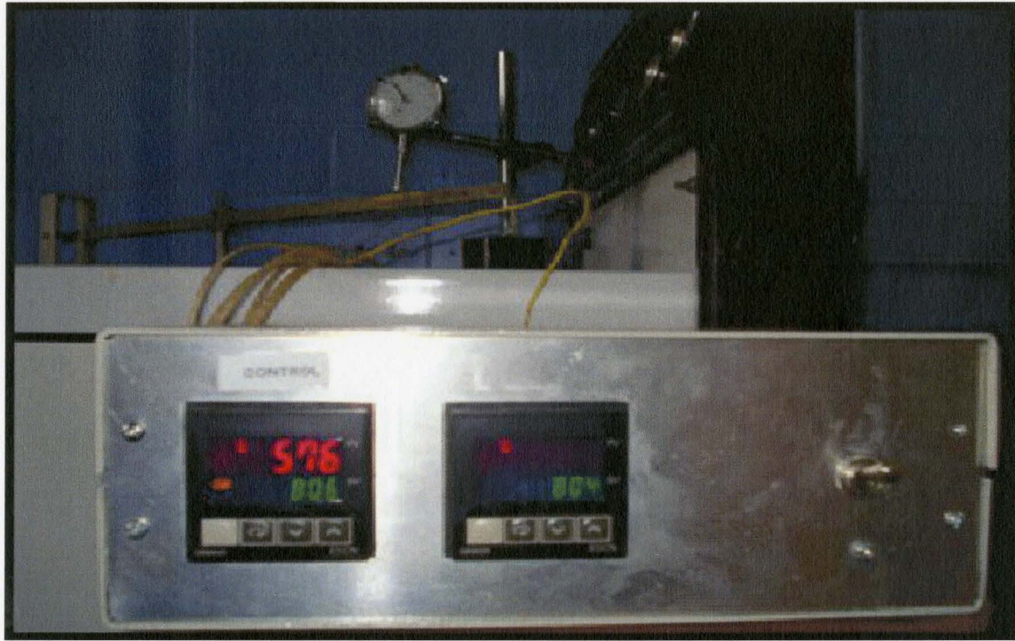
Figure 2.4. External temperature controller used in the experiments.
