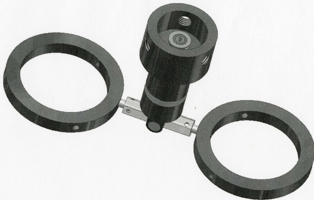
Figure B.1: Stereo head CAD drawing
