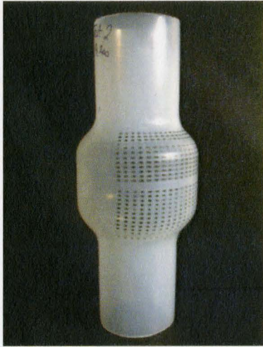
(a) Tube didn't form the shape of the die (Case 1)
