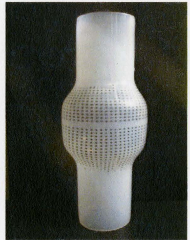
(f) Part shape conforms to the die shape (Case 6)
