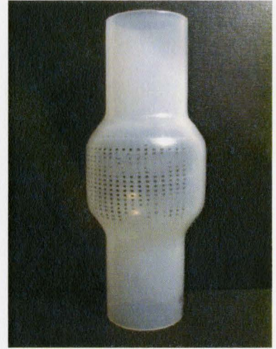
(c) Tube buckling initiation (Case 3)
