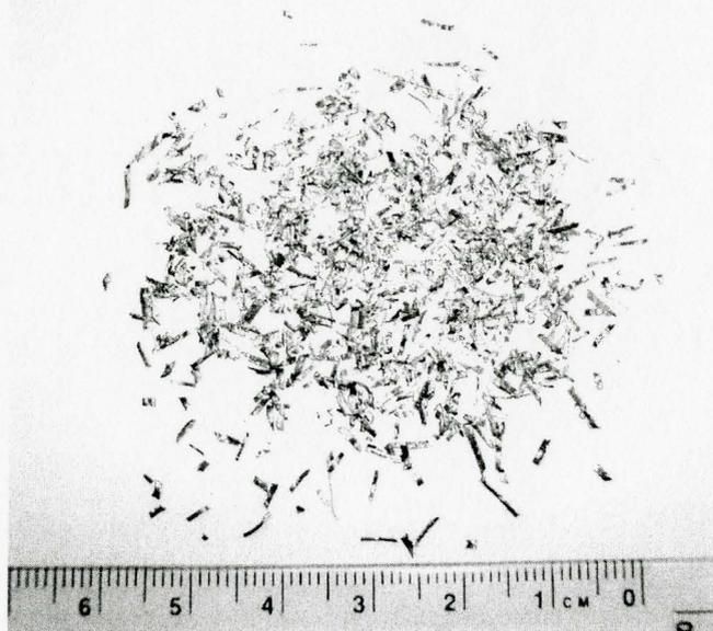
Figure 2.30  $\text{Cu}_{43}\text{Zr}_{43}\text{Al}_7\text{Ag}_7$  alloy ribbons after hot pressing operation.
