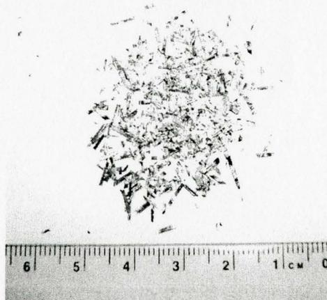
Figure 2.11 Melt spun ribbon of  $\text{Cu}_{43}\text{Zr}_{43}\text{Al}_7\text{Ag}_7$ .
