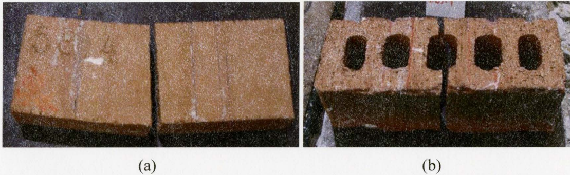
Figure 5.5 (a) Small Scale MOR Failure Mode (b) Full Scale MOR Failure Mode
