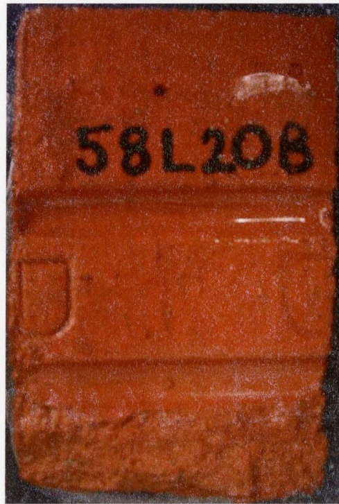
Figure 5.35 Specimen FL20 Flawed Edge After 65 F/T Cycles
