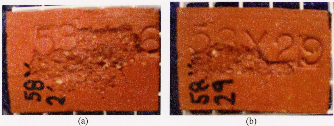
Figure 5.25 Mass Loss for Specimens (a) X26 and (b) X29 at Cycle Number 100
