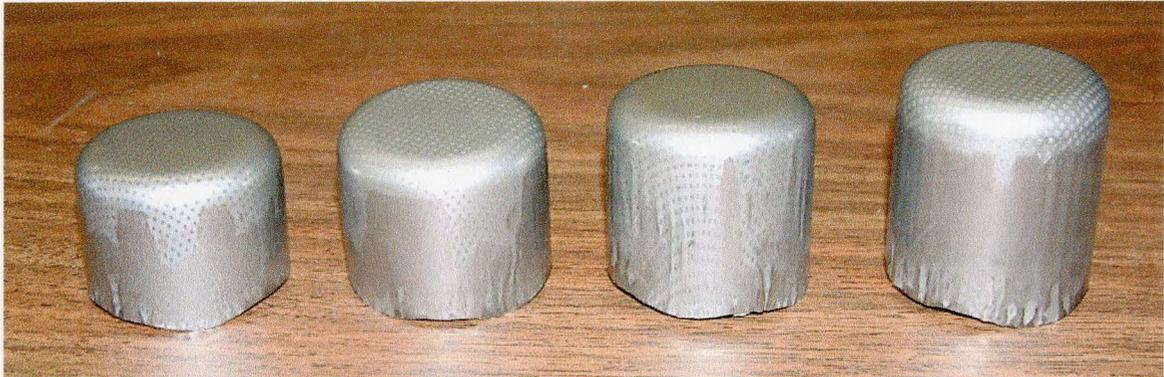
Figure 5.7 Redrawn cups from four deep drawn cups with different initial diameters: from left to right, 95 mm, 100 mm, 105 mm, 110 mm respectively
