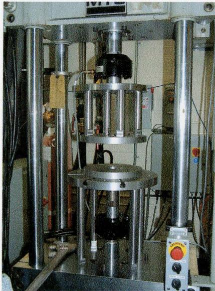
Figure 2.4 Deep drawing equipment: modified tensile testing machine
