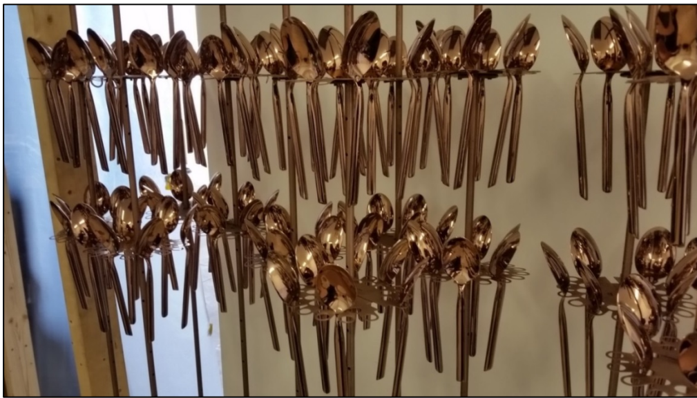
Figure 29: Mounting racks for coating utensils.
