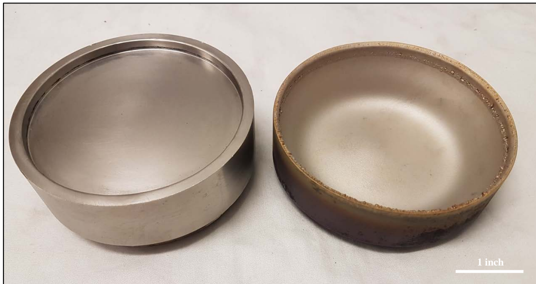
Figure 23: New (left) versus depleted (right) titanium cathode targets.
