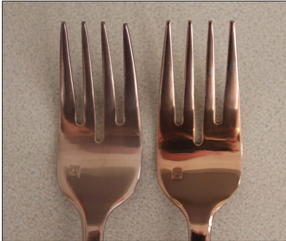
Figure 26: Texture comparison of sample A12 (left) with a sample from a typical deposition cycle (right). Notice the significant difference in reflection.
