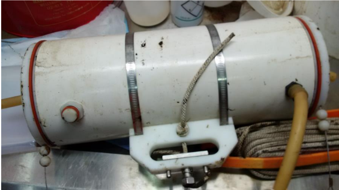
Figure 3.3- the sampling Van Dorn used in summer 2016 for weekly geochemical data sampling.
