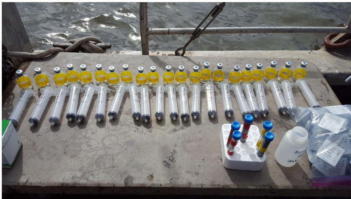
Figure 3.6- the sampling table for the FIS. Each depth had it's own syringe, needle and bottle to make sure there was no cross contamination when handling 20 samples at once.
