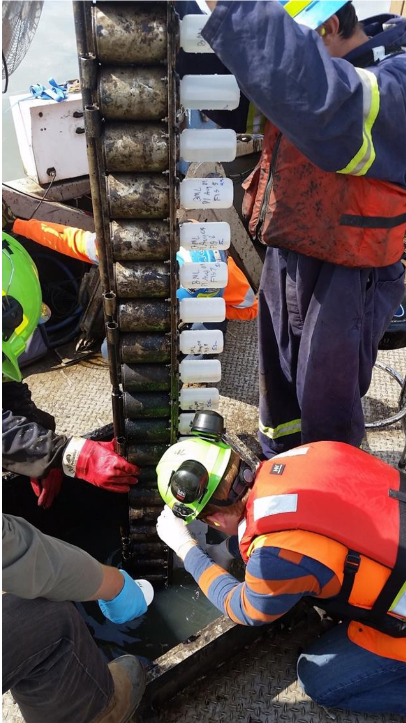
Figure 3.4- As the FIS was drawn up one sample chamber at a time, HDPE bottles were screwed on to minimize sample loss.
