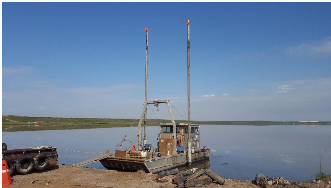
Figure 3.7- the specialized Fixed-Interval Sampling boat used for both FIS days in August.
