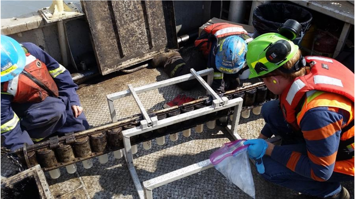
Figure 3.5-The sampler had to be placed horizontally to ensure all water sample chambers were properly evacuated and the pressure system did not force the HDPE bottles off of the threading.
