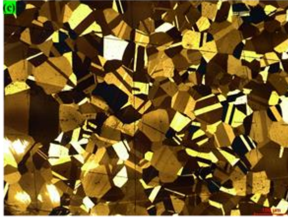
Figure 4.8. Grain size evolution in samples of a) Fe-30Mn, b)Fe-30Mn-0.03Nb and c)Fe-30Mn-0.05Nb after holding for 8 days at 1000°C
