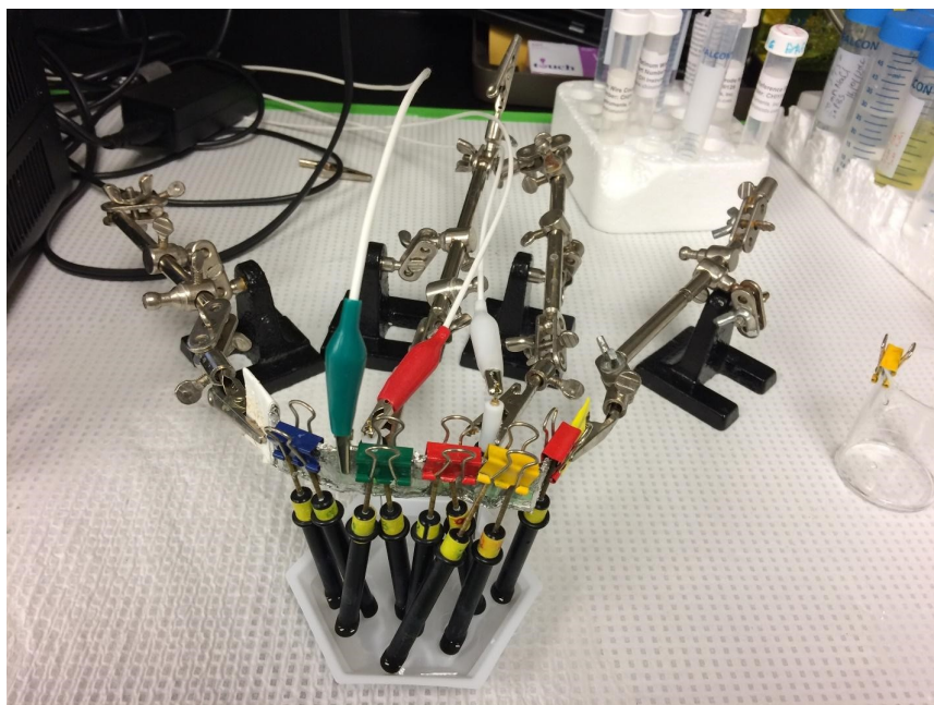
FIGURE 2.6: Multiple electrodes can be electrochemically cleaned together. This should be followed by performing H_2SO_4 scans per individual electrode. The electrode holder seen above is created with aluminum foil, clips and tape, held by two helping hands.
