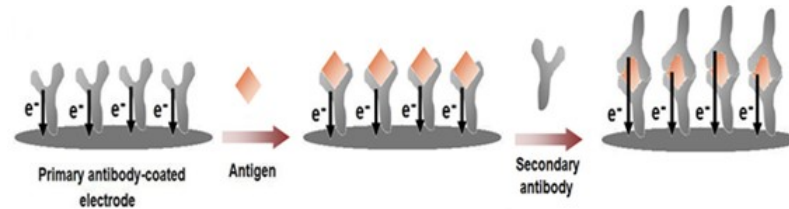
FIGURE 1.7: Schematic illustration for the label-free voltammetric immunosensors. The primary antibody is coated on the electrode surface, and the electro-active residues in the antibody structure give a specific current response. Upon the binding of the target antigen with the antibody, the specific current response of the antibody layer changes. This change can either be an increase or a decrease depending on the structure of the antigen and the conformational changes that would occur upon the formation of the antigen-antibody complex. Then, the current responses would be further altered with the binding of the secondary antibody, which would also contribute to the current response with its intrinsic electro-activity. Adapted from reference [41] with the permission from the Molecular Diversity Preservation International.
