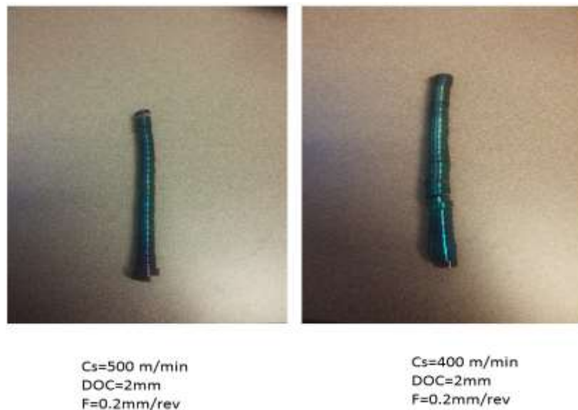
Fig 9) Hard to break chips generated from AISI 1045
