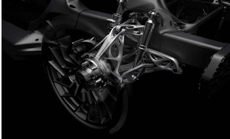
Figure 12 The Blade's 3D metal printed suspension assembly (Divergent 3D, n.d.).
