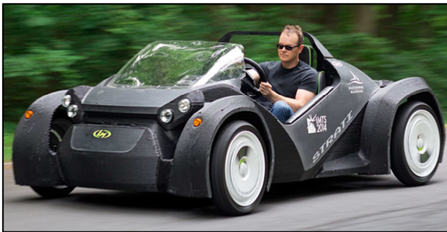
Figure 5 A prototype of LM's first 3D printed car, the Strati (Stains, 2015 in Dyer, 2015).
