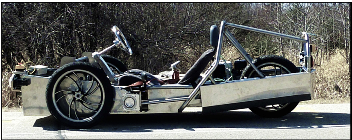
Figure 4 Urbee's tubular, alloy-steel sub-frame (Kor Ecologic, 2014).
