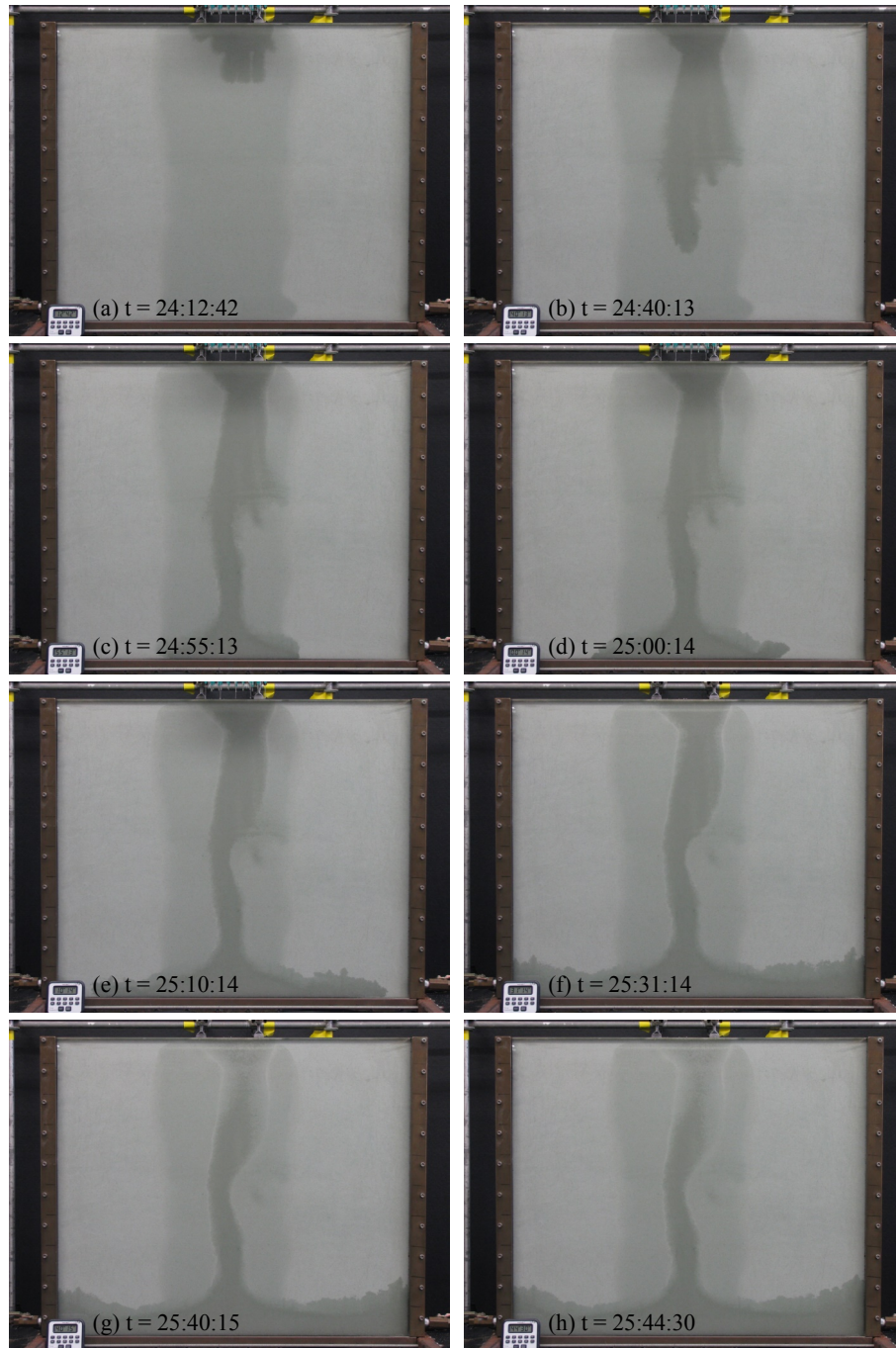
Figure 3.6. The ethanol-water boundary zone of lower saturation (halo effect) in experiment CF-J. The sequenced photographs begin with time zero being the beginning of ethanol application (a) t = 24:12:42 , (b) t = 24:40:13 , (c) t = 24:55:13 , (d) t = 25:00:14 , (e) t = 25:10:14 , (f) t = 25:31:14 (application of water stopped at 25:30:00), (g) t = 25:40:15 , and (h) t = 25:44:30 .
