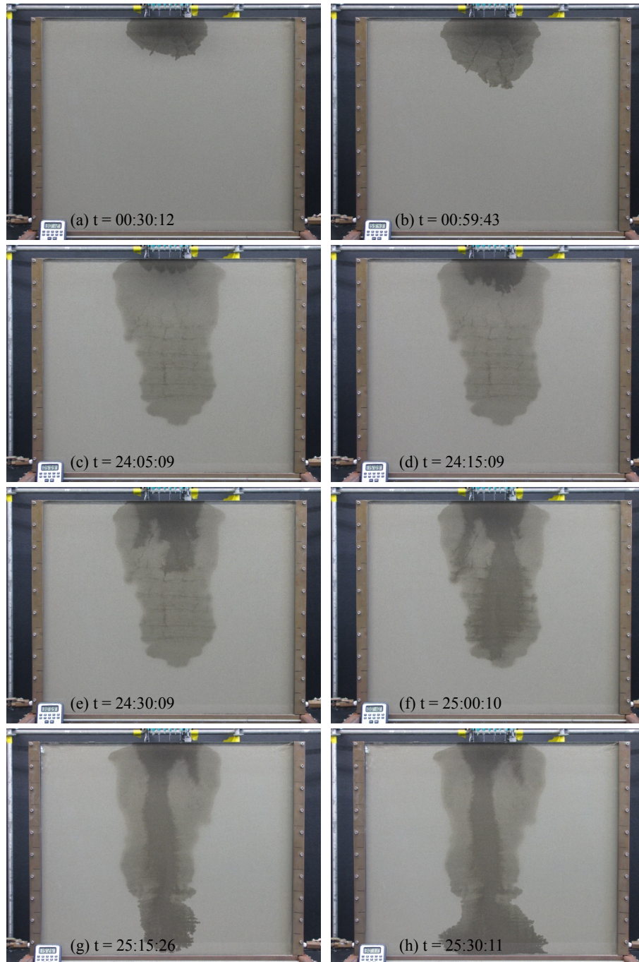
Figure 3.14. Water following ethanol infiltration constant flux experiment CF-E exhibiting two unstable displacements resulting in two focused flow events. Sequenced photographs of experiment CF-E with time zero being the beginning of ethanol application (a) t = 00:30:12, (b) t = 00:59:43, (c) t = 24:05:09 (start of water application), (d) t = 24:15:09, (e) t = 24:30:09, (f) t = 25:00:10, (g) t = 25:15:26, and (h) t = 25:30:11.
