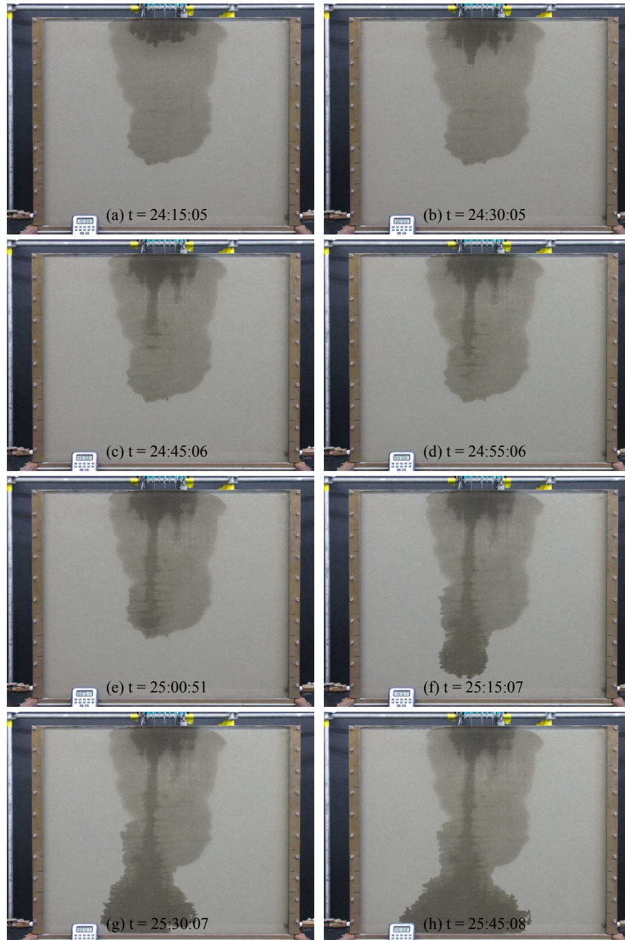
Figure 3.12. Water following ethanol infiltration constant flux experiment CF-D exhibiting minor heterogeneity. Sequenced photographs of experiment CF-D with time zero being the beginning of ethanol application (a) t = 24:15:05 (start of water application), (b) t = 24:30:05 , (c) t = 24:45:06 , (d) t = 24:55:06 , (e) t = 25:00:51 , (f) t = 25:15:07 , (g) t = 25:30:07 , and (h) t = 25:45:08 .
