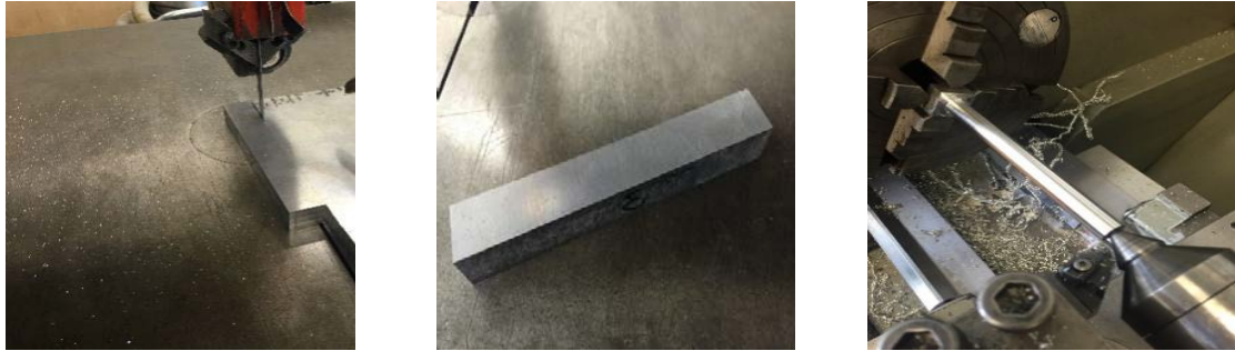
Figure 3.2. Cutting and machining of AA7075-T6 plate stock into cylinders for obtaining cylindrical test specimens.
