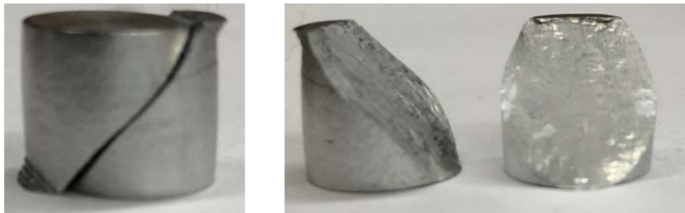
Figure 5.48. The slant failure of a T6 temper cylindrical specimen tested at room temperature.
