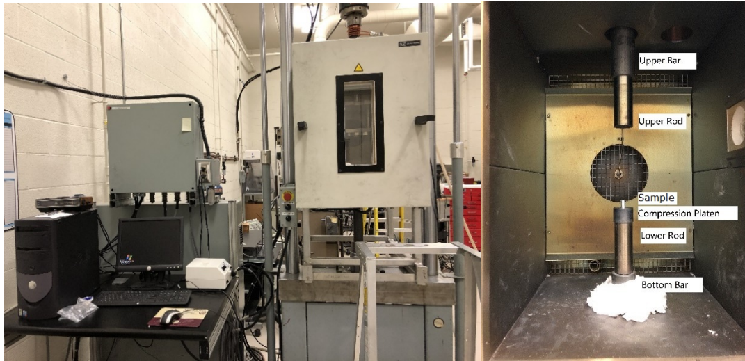
Figure 3.6. MTS servo-hydraulic mechanical test system for hot uniaxial compression experiments. Image on the right shows the inside view of the environmental chamber with upper and lower loading arms. A cylindrical test specimen is also shown above the bottom compression platen.
