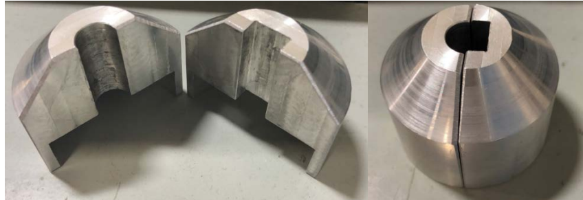
Figure 3.7. Two different views of the fixtures for centering of the cylindrical and cubic specimens on the bottom compression platen.
