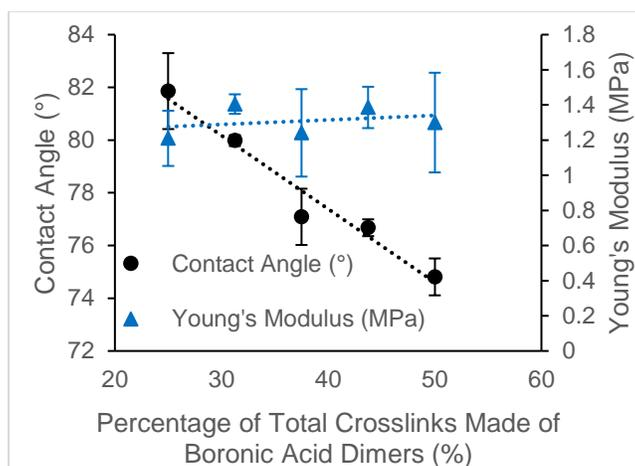
Figure 21. Physical properties of silicone boronic acid elastomers as a function of varying crosslink type.
