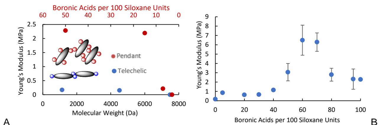
Figure 17 Moduli of Silicone Boronic Acid Elastomers A: homopolymers telechelic SiBA-17 and pendant SiBA-P50, B: mixtures of telechelic SiBA-17 when diluted with pendant SiBA-P7.
