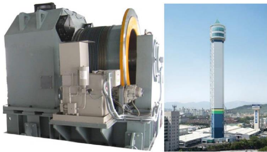
(a) 9-phase PMSM lift drive machine and the elevator test tower [24].
