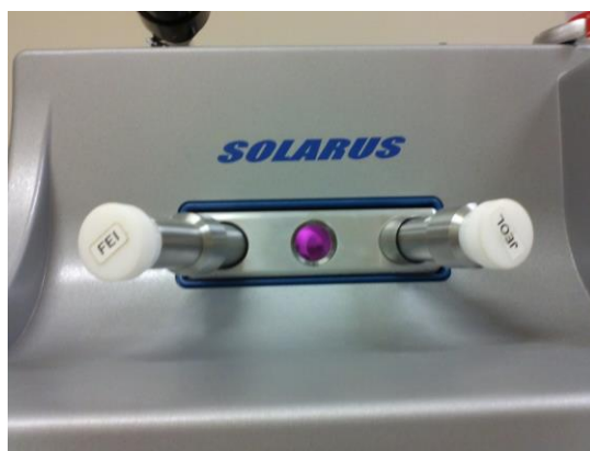
Figure A.1.1 N 2 /H 2 plasma activated in the Solarus 950 Gatan Advanced Plasma System. The central window shows the pink colour of the plasma inside the chamber.
