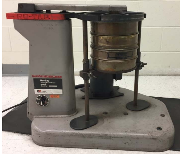
Figure 51: Ro-Tap sieve shaker at McMaster University
