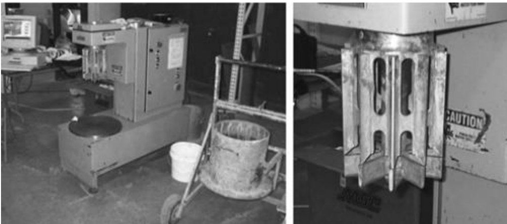
Figure 1.13: BML viscometer (left) with an enlarged view of inner blades (right) (American Concrete Institute, 2008)
