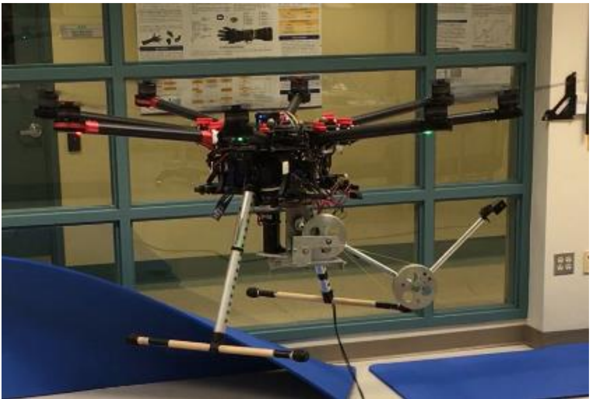
Figure 10.1: Aerial Manipulator: DJI S1000 octo-copter integrated with a 3 DOF robotic manipulator during a test flight
