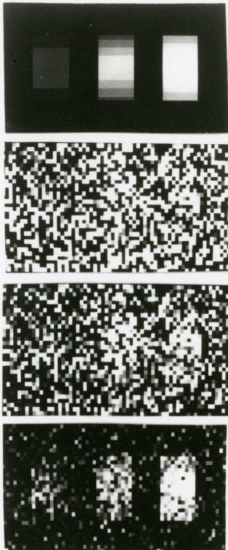
FIGURE 3.6 Simulated TPA images for elliptical cylinders of bone with thicknesses from left to right of 0.6, 1.0 and 1.4 g/cm<sup>3</sup>. The images from top to bottom are with no statistical noise, with transmitted count rates of 500, 5000 and 50,000 per pixel in the high energy channel.
