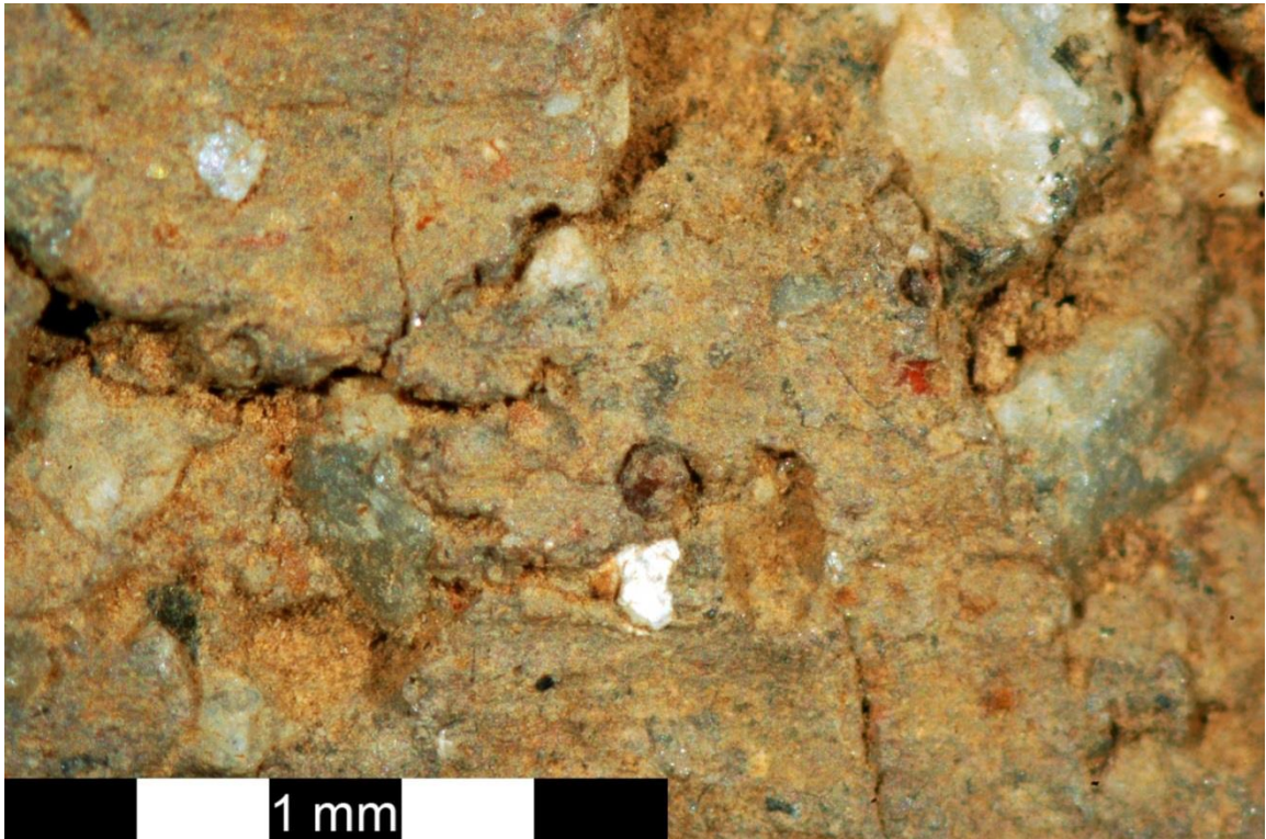
Figure 32: Microscope photo of a paste containing Bluish-Grey Quartz temper. The bluish-grey particles are abundant in this sample. Note also the presence of an iron oxide particle and a lack of obvious feldspar.
