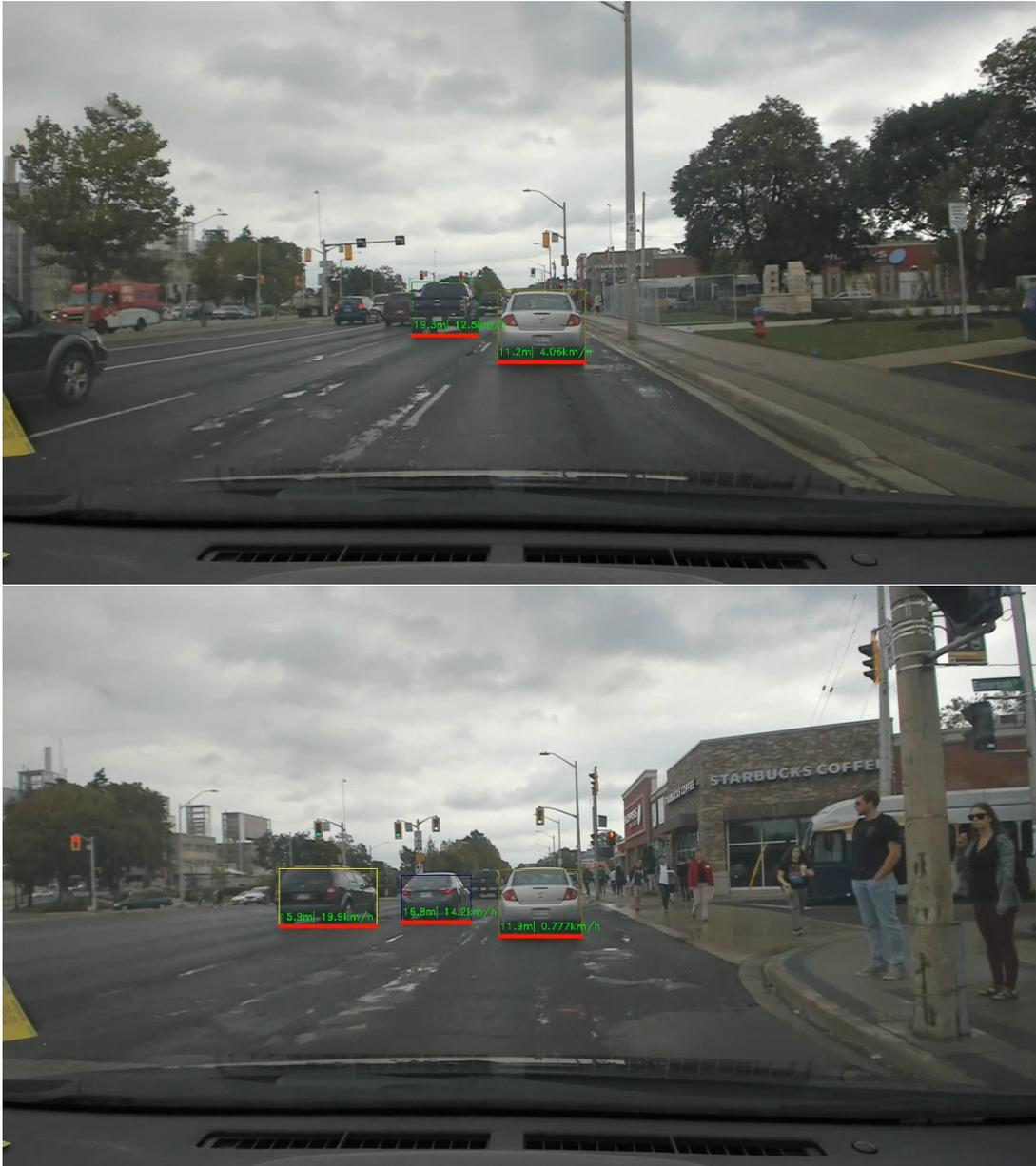
Figure 4.7: Sample result of estimated distance and longitudinal speed to frontal vehicles (better view in color).
