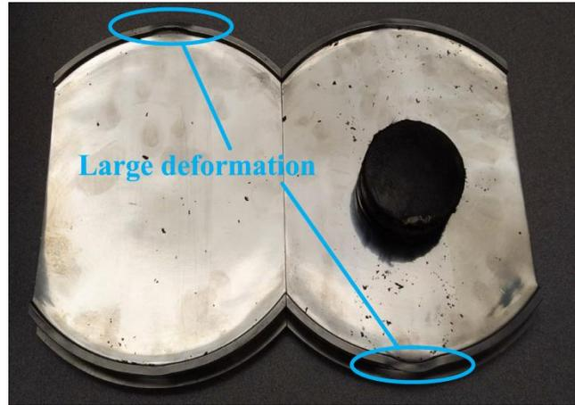
Figure 3-14 Inspection of Specimen C after test (two plates from north isolation bearing)
