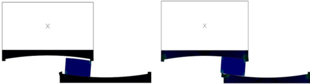
Figure 2-3 Different failure behaviors of double friction pendulum (left: due to uplift; right: due to yielding)
