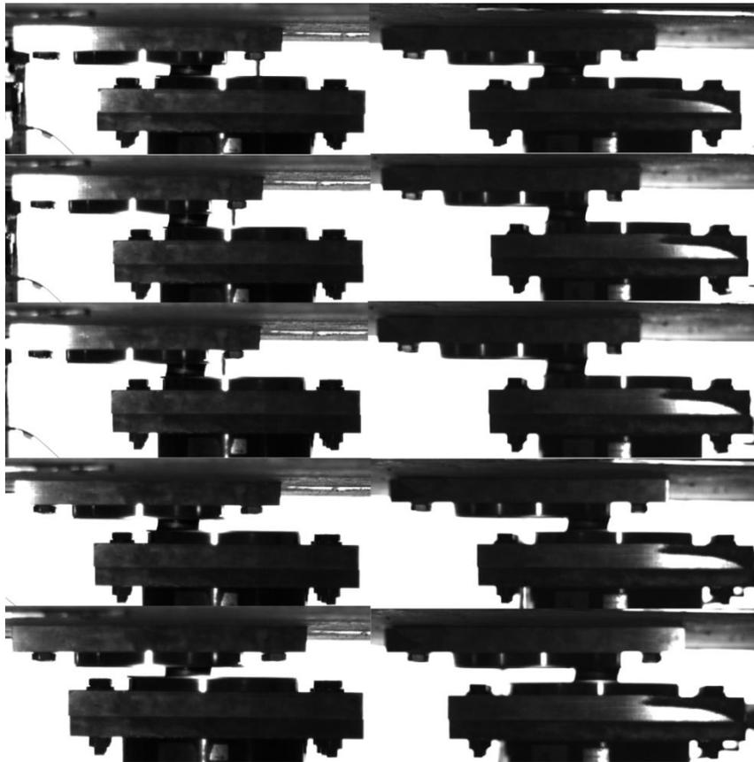
Figure 3-11 Specimen B at increasing time steps under 135% baseline motion (left column: south bearing, right column: north bearing)
