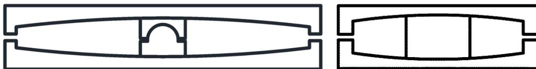
Figure 1-3: Double friction pendulum bearing with different inner sliders (left: articulated slider; right: non-articulated slider)
