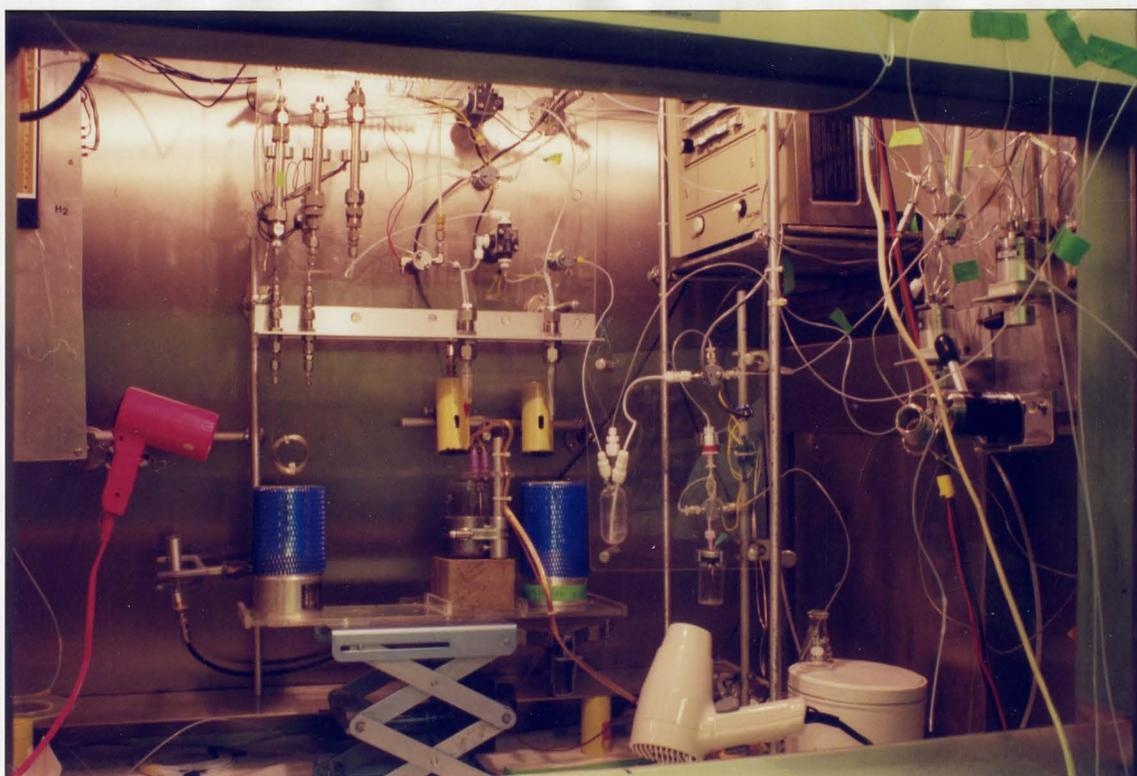
**Figure 29:** Apparatus for  $^{11}\text{C}$ -Acylation Reactions
