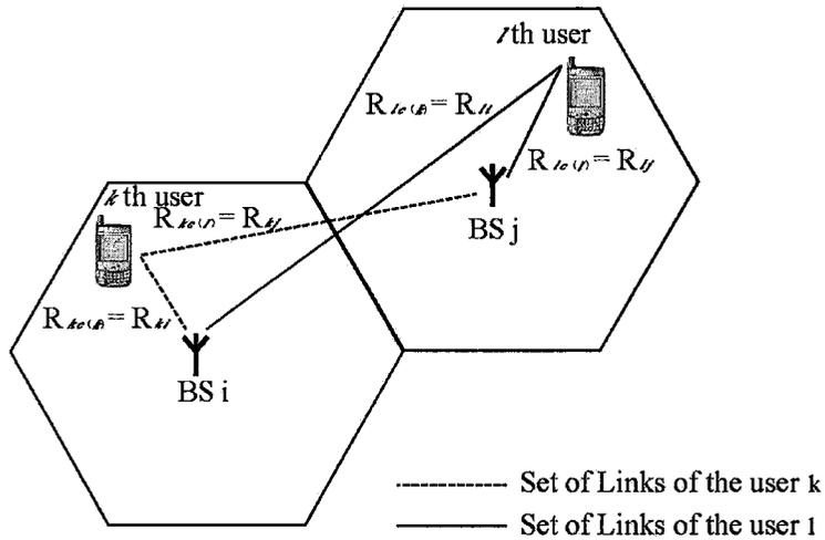
Figure 2.4: Downlink Channel Correlation Matrix Model
