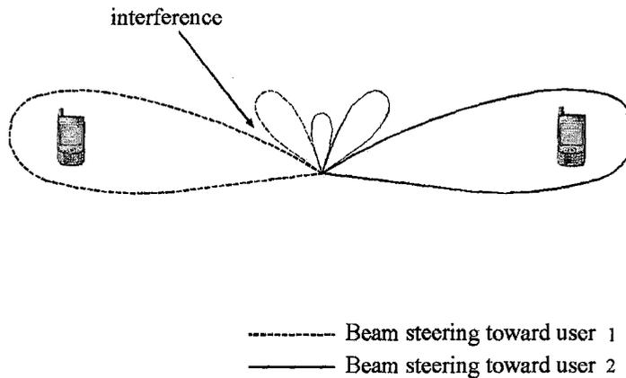
Figure 2.3: Beamforming Illustration
