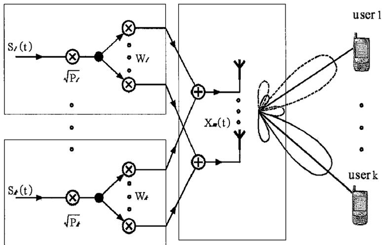
Figure 2.5: Downlink Beamforming Structure Illustration
