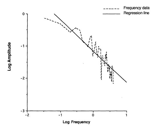
Figure 3. The same frequency data of figure 2, replotted after logarithmic transformation and regression analysis to determine line of best fit.
