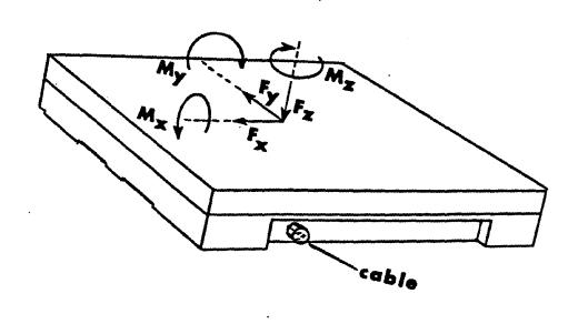
Figure 1: Orientation of ground reaction forces and moments measured from the force platform. Taken from AMTI manual, 1985.
