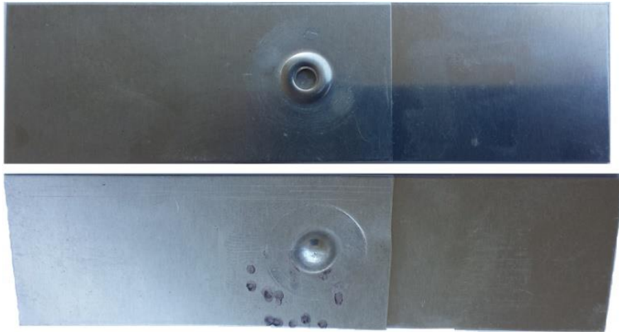
Figure 6.9. Photographs of a successful hot clinched joint. The clinching conditions were 7.5 kA, 3 sec, and 60kN.
