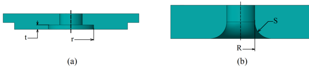
Figure 5.4. Two different blank holder designs utilized in the FE simulation of die-less clinching, (a) stepped edge blank holder and (b) round edge blank holder.
