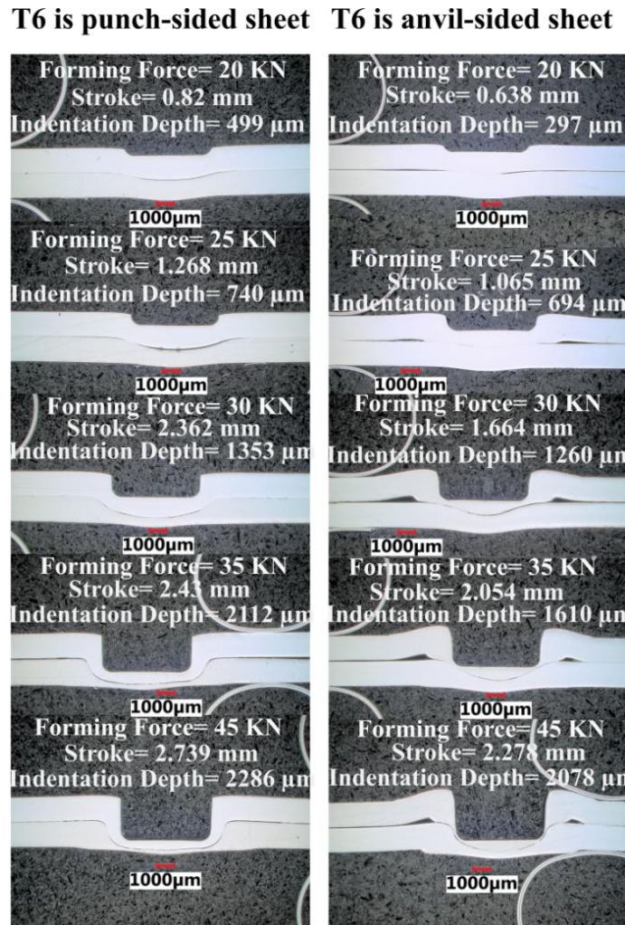
Figure 3.12. A set of optical images of the cross-sections through die-less clinch joints formed in O and T6 tempers. The left and right columns present the case of T6 temper sheet on the punch-side and anvil-side respectively.
