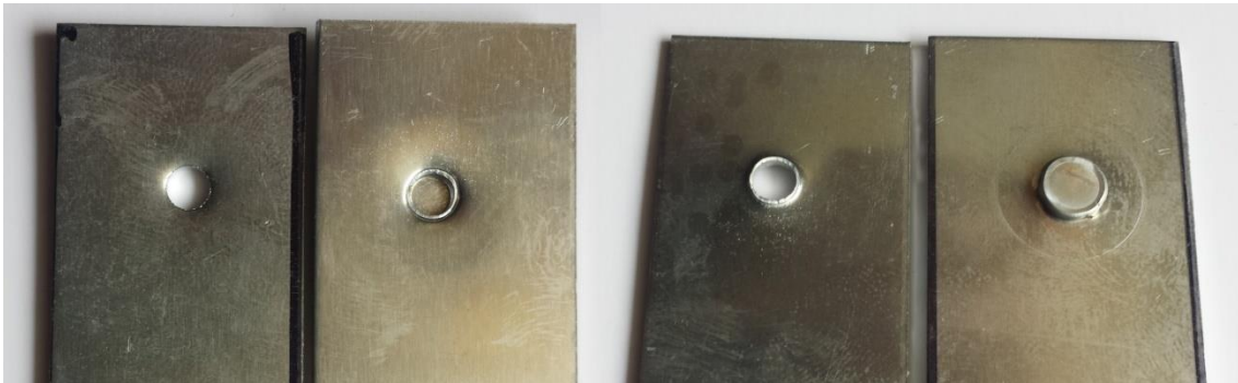
Figure 2.25. Unbuttoning failure mode of the clinched joint. The first two photos on the left show the upper surface of the punch-sided and die-sided sheets respectively. The photos on the right show the lower surface of the punch-sided and die-sided sheets respectively.
