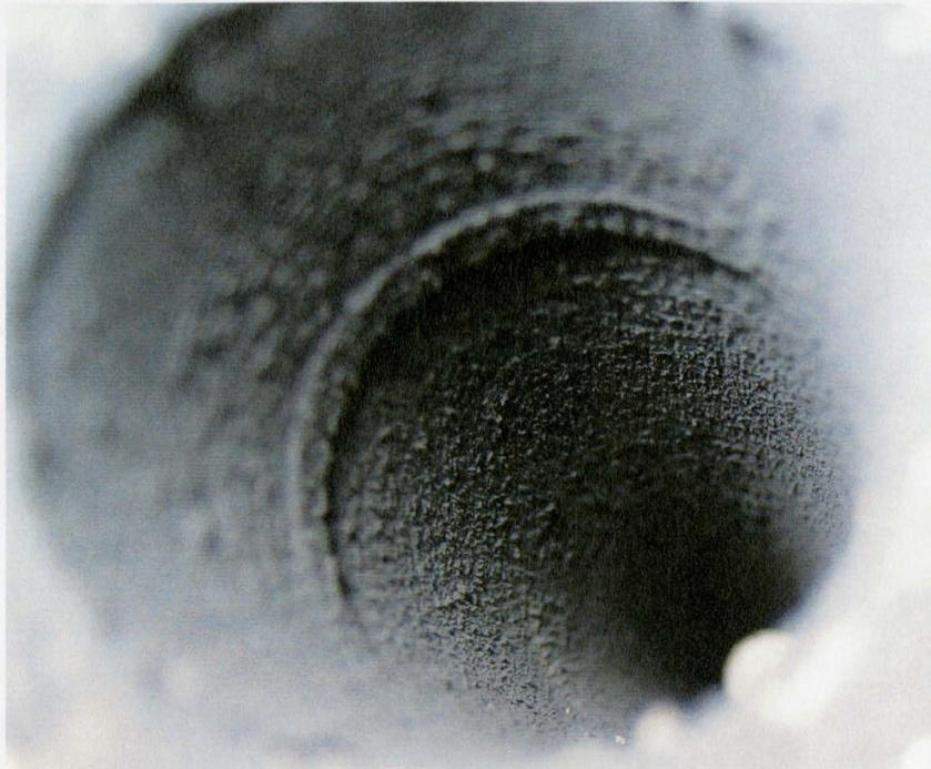
Figure C.2: Digital image bottom of the portion inside the CWCS gas channel at upstream exposed to diesel exhaust gas for 2 hrs at an initial coolant temperature of 20 degrees celcius
