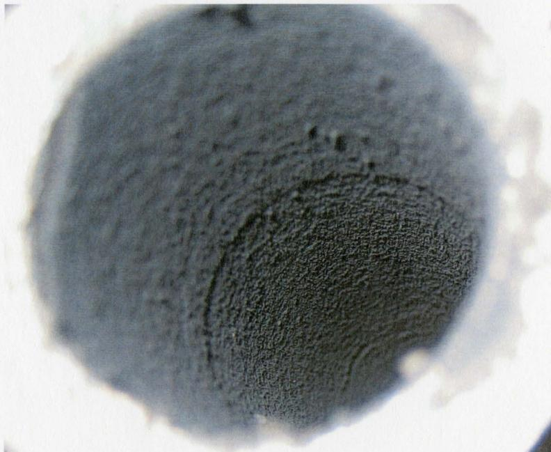
Figure C.3: Digital image of the top portion inside the CWCS gas channel at downstream exposed to diesel exhaust gas for 2 hrs at an initial coolant temperature of 20 degrees celcius
