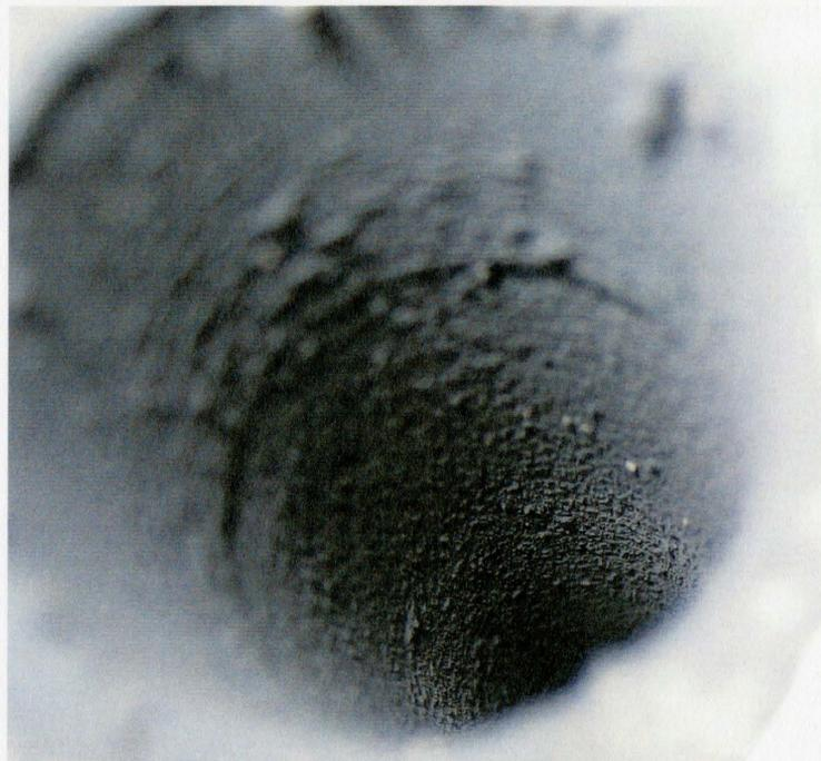
Figure C.1: Digital image of the top portion inside the CWCS gas channel at upstream exposed to diesel exhaust gas for 2 hrs at an initial coolant temperature of 20 degrees celcius
