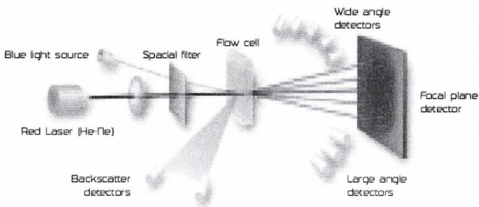
Figure 3.2.2 Structure Scheme of Mastersizer (Image from Malvern Instruments Online Brochure, <http://www.malvern.co.uk>)
