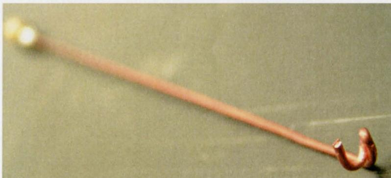
Figure B.2.4 – The fork shaped hook used for probe #7.
