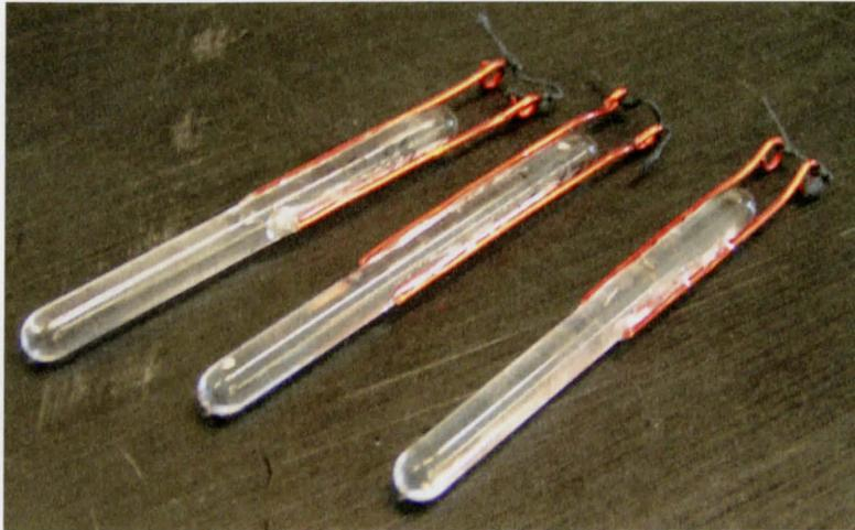
**Figure B.1.6 – Probe #6. 5mm diameter glass rods with a rounded tip and suture string tied across the top**
