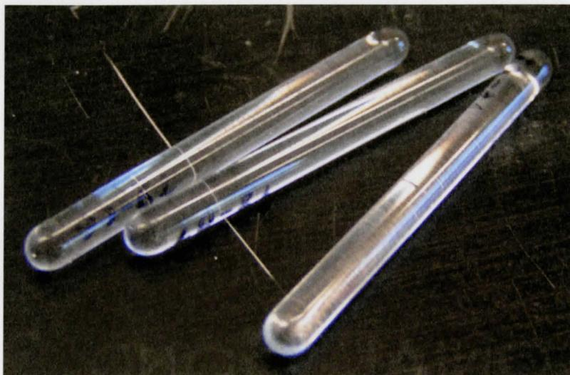
**Figure B.1.3 – Probe #3. 5mm diameter glass rods with a rounded tip**
