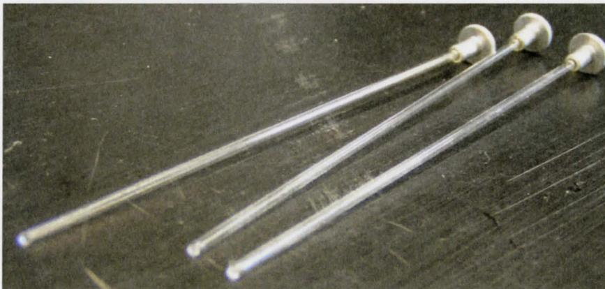
**Figure B.1.8 – Probe #8. The final form of the probe. A capillary tube with a flat head glued to the top for easy lifting**
