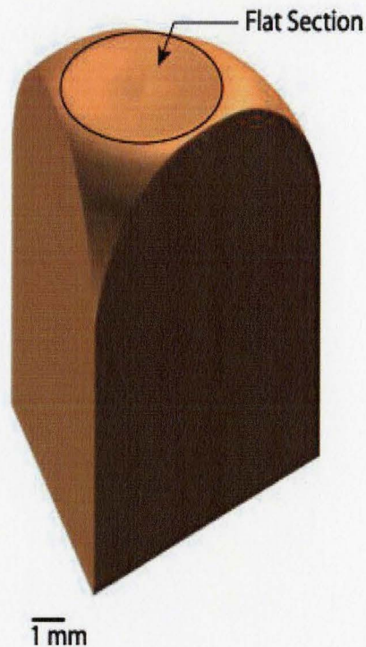
Figure 5-10: 3D Image of Tool Wear Pattern
