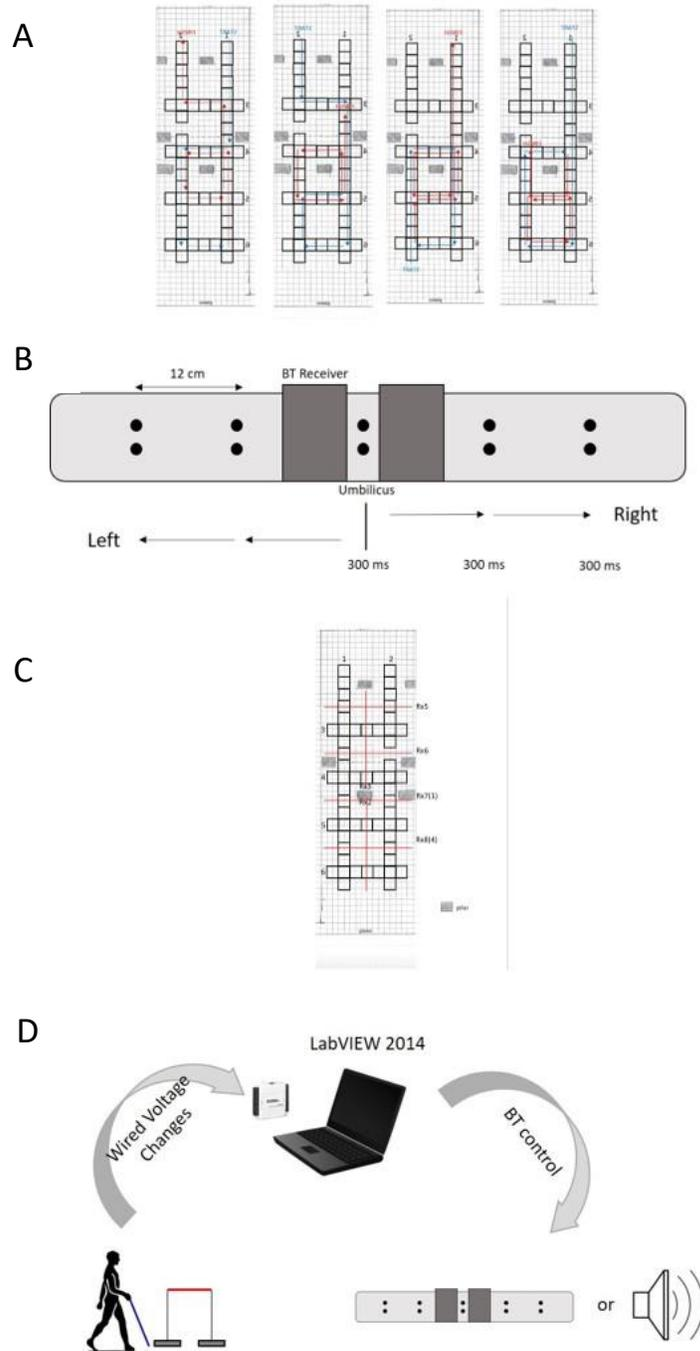
**Figure 1.** Experiment Overview. A) Four routes equalized for difficulty (10 turns, ~127 ft in length). B) Schematic of vibrotactile navigational belt. Vibrotactile sweeping sensation begins from the umbilicus and moves towards the left or towards the right (as indicated by the arrows). C) Laser transmitter/receiver grid. D) Systems overview during experiment.
