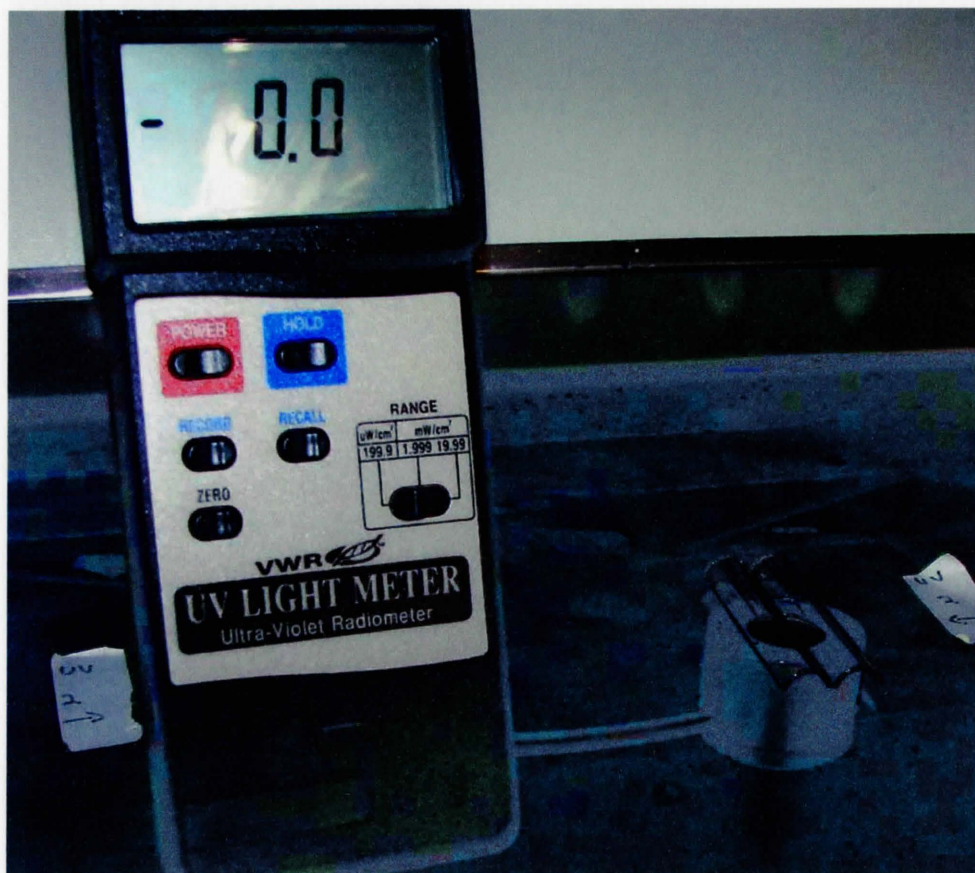
Figure 2.6 Measurement of UV intensity in the glass tube.
