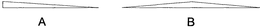
Figure 5.4: Examples of degenerated triangular elements: (A) Small edge length. (B) Small area.
